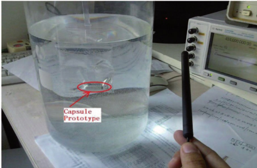
Fig. 19 Capsule endoscope prototype with designed 400 MHz transceiver in emulated environment
