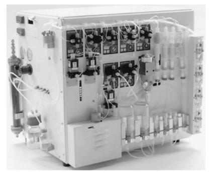
FIGURE 7-4. An automated <sup>18</sup>F-FDG synthesis box, Explora-FDG4, manufactured by CTI Molecular Imaging, PET NET. (Courtesy of CPS Innovations, Knoxville, TN, USA.)
