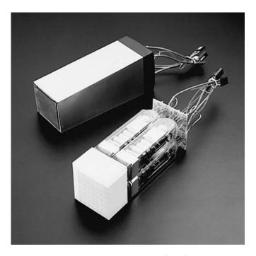
FIGURE 2-3. A typical commercial block detector  $(8 \times 8)$  attached to four square PM tubes (bottom) and a packaged module (top), developed and manufactured by CPS Innovations. (Courtesy of CPS Innovations, Knoxville, TN, USA.)
