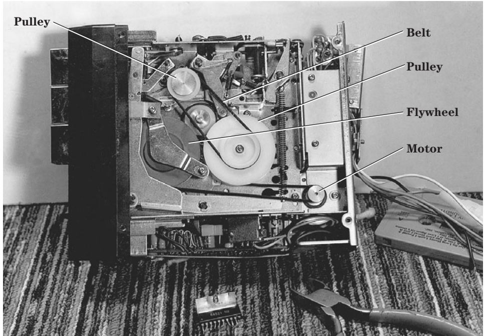
5-5 Clean up all drive belts, idlers, and pulleys for slow speeds.
