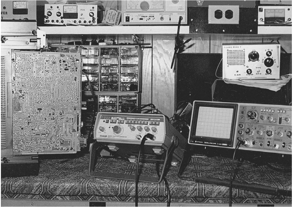
2-2 The oscilloscope can quickly check critical waveforms within an electronic chassis.
