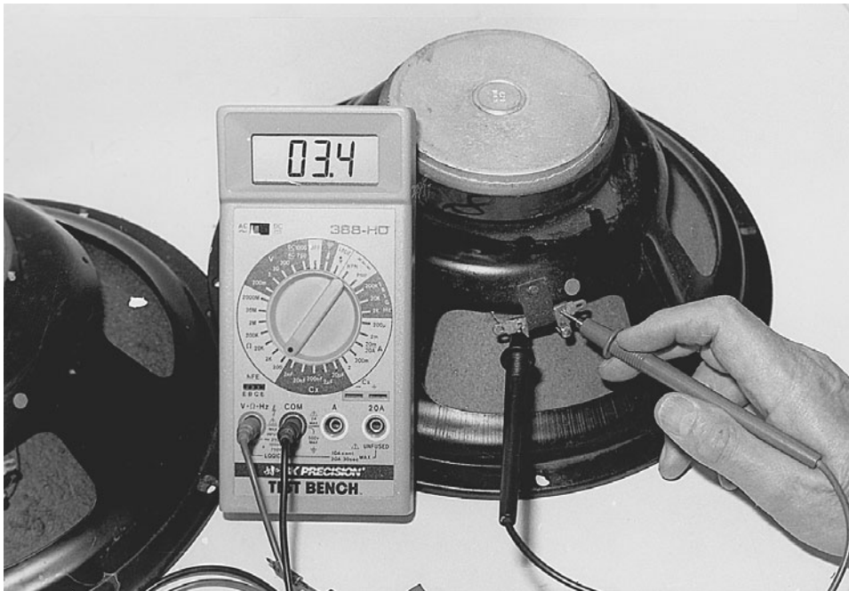
4-33 A 15-in 4-ohm speaker tests only 3.4 ohms on the DMM.
