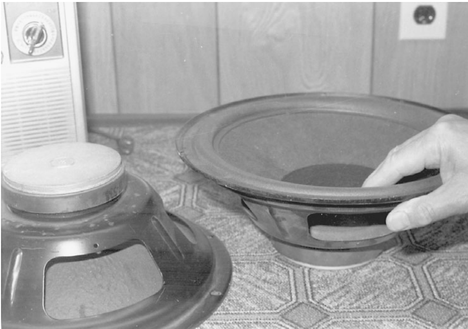
9-35 Push up and down on the large speaker cone to see if the voice coil is dragging or frozen.
