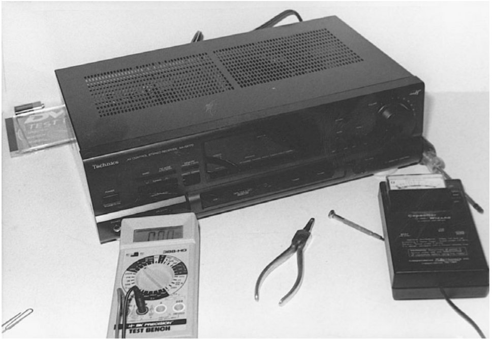
10-31 Take critical voltage measurements on the LCD driver IC for no display.
