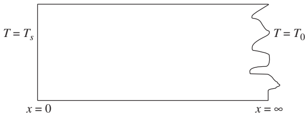
FIGURE 9.6 Semi-infinite medium with initial temperature at T_0 .
