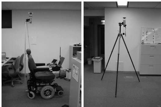
Fig. 4. Image acquisition device of the powerwheel and the tripod type
