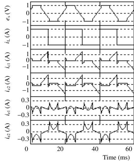
Fig. 8. Simulation results when the power supply frequency has no fluctuation, and the power supply voltage distorts.
