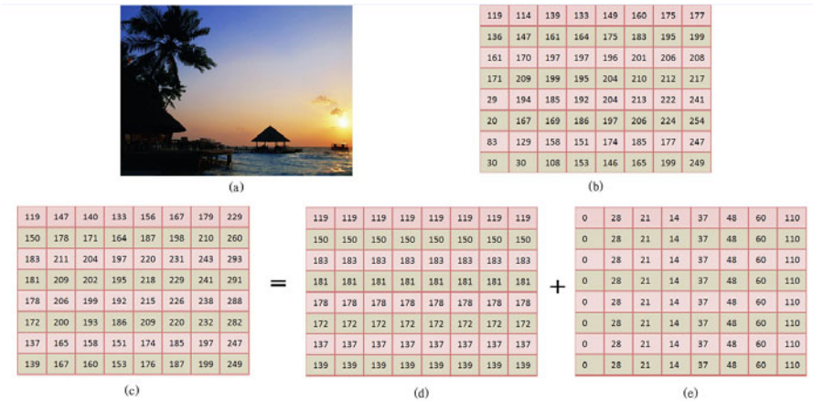
Fig. 3. The process of the proposed algorithm.(a) source image,(b) I , (c) I' ,(d) A' ,(e) B' .
