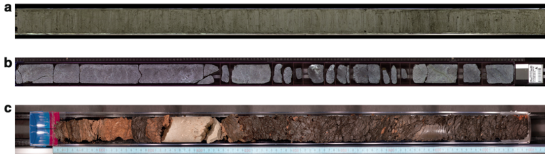
Ocean Drilling, Figure 4 Core sample photographs. A few examples from a vast collection of legacy cores since DSDP openly available to scientists from core repositories. a Exp. 302 M0004-11 \times (297.30–301.35 m; ~49 Ma): there is an extremely dense concentration of remains of the hydropterid (freshwater) fern Azolla – unprecedented in other Eocene sections yielding Azolla . The event testifies to an extreme change in environmental conditions at the base of the lower middle Eocene (Lutetian) (from Proc. IODP 302, 2006). b Exp. 312 1256D-223R (1450.78–1452.28 mbsf): gabbro (lower crustal rock) section first recovered from the Pacific Ocean after ODP Leg 206 and IODP Exp. 309 at Hole 1256D. c Exp. 343 C0019-17R (821.5–822.5 mbsf): strongly deformed clays inferred to be the slip zone (decoupling) of the 2011 Tohoku earthquake fault (Proc. IODP 343, 2013) (This photo was taken before cutting into halves (from CDEX, JAMSTEC)).
