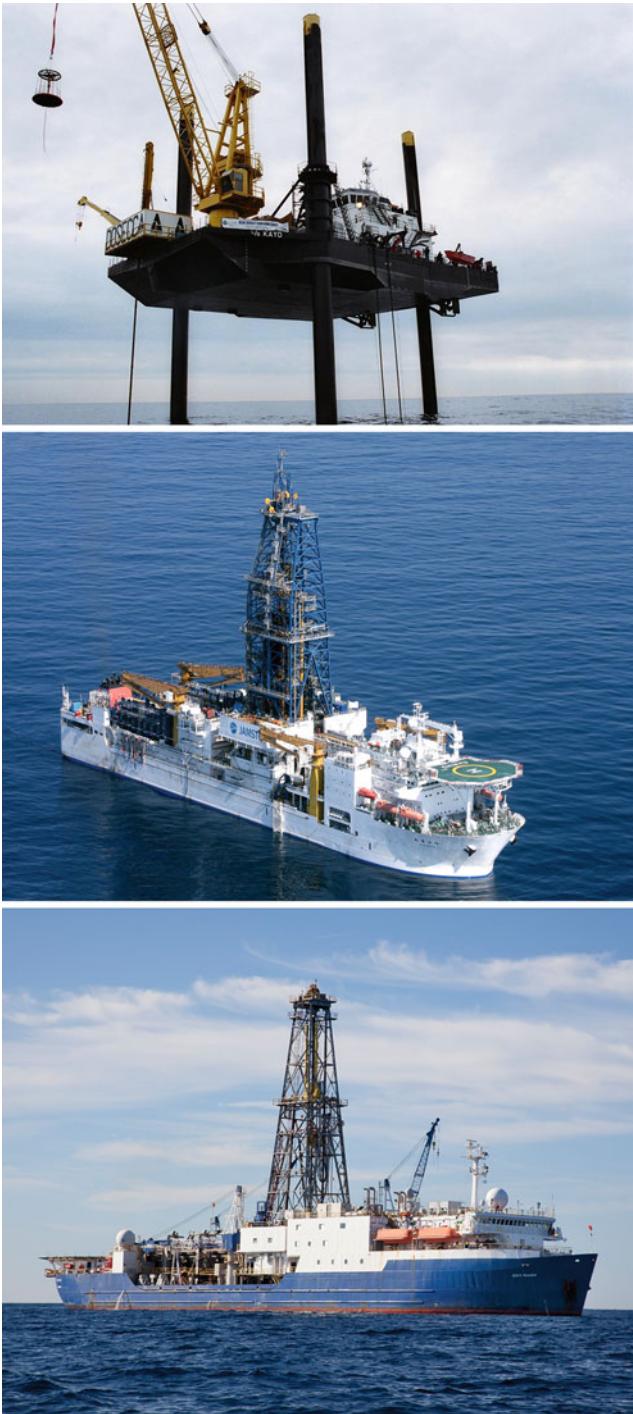
Ocean Drilling, Figure 2 Drilling platforms utilized in the current IODP program (see Table 1). JOIDES Resolution has been operating since the start of ODP. Chikyu operated by Japan Agency for Marine-Earth Science and Technology is a new addition with long-awaited riser drilling capability suitable for deep drilling. Mission-Specific Platform charters are an operationally optimal platform for drilling not suitable for JR or Chikyu , such as ice-covered or shallow waters.
