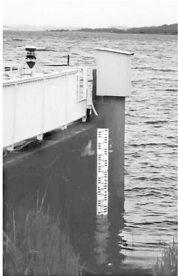
Sea-Level, Figure 3 Tide gauge in a harbor site with GPS setup at a tripod (left).
