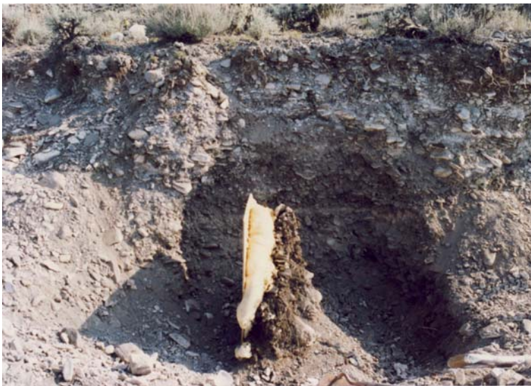
Figure 2A.48: Soil monolith collected from the post-1983 colluvial wedge shed from the Borah Peak, Idaho, fault scarp. Shown from left to right, the plywood board, the urethane foam (yellow), and the monolith. The monolith soil is darker because it was sprayed with an aerosol clear fixative. Subsequent to this photograph, the standing monolith was secured by wrapping it in rubber carpet padding. The base was then cut away and the monolith was detached and laid down for transport. Photo by J. P. McCalpin, 1985.
