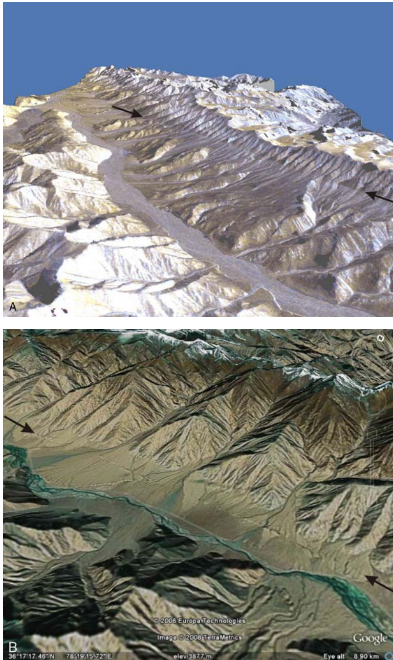
Figure 2A.5: Three-dimensional perspective view of Karakax valley (northwestern Tibet). (A) from a DEM created by interferometry from two radar images (center at 36.1^{\circ}\text{N} latitude, 79.2^{\circ}\text{E} longitude). Scale varies in this perspective view, but the area is about 20 km (12 miles) wide in the middle of the image, and there is no vertical exaggeration. Elevations range from 4000 m (13,100 ft.) in the valley to over 6000 m (19,700 ft.) at the peaks of the glaciated Kun Lun mountains running from the front
