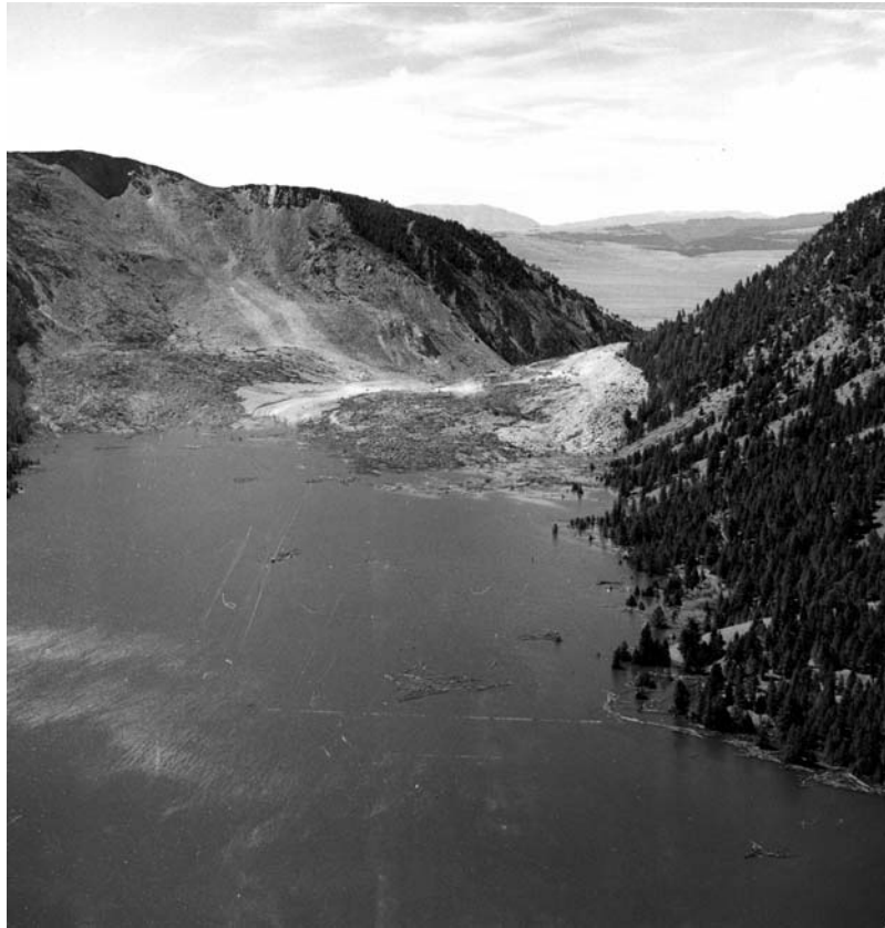
Figure 8.1: Madison Canyon landslide, triggered by the 1959 Hebgen Lake, Montana, earthquake ( M_w 7.1). Strong shaking caused 28 \times 10^6 \text{ m}^3 of rock to slide into the canyon, which dammed the river and created a lake more than 60 m deep (Hadley, 1964). Slide scar at left is 400 m high, debris is as thick as 67 m in valley axis, and slide debris traveled 130 m up the right valley wall. Twenty-eight people were killed by the slide. [Photograph courtesy of J.R. Stacy, U.S. Geological Survey Photographic Library (photo no. 209a).]
