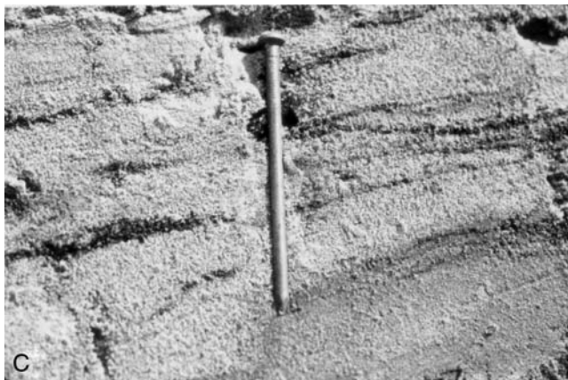
Figure 7.19: Sand dikes and sills exposed in a nonliquefiable cap of silt and clay; the dikes and sills are interpreted as having originated by liquefaction during the 1811–1812 New Madrid earthquakes. Outcrop is the bank of a ditch in the meizoseismal area of the 1811–1812 earthquakes. (A) Overview and line drawing of typical small dikes and small sills. The sill extends far beyond the photograph and is at least 25-m long. Rectangle shows area of part (B). (B) View showing details of layering in sills. (C) Very close view showing details of layering in sill. Sill consists of fine- and medium-grained sand with some silt- and sand-sized lignite. Black bands are laminae of small pieces of lignite.
