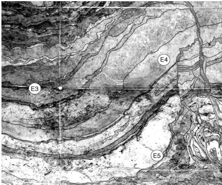
Figure 6.40: Photomosaic of the main fault zone on the south wall of trench T2, cut 2, at Hog Lake, showing evidence for paleoearthquakes E3–E5; individual photos are 1 m 2 . Note the angular unconformities associated with earthquakes E3 (upper left center) and E5 (lower right center). Earthquake E4 is represented by a clear upward termination (upper right center) and mismatch of units across that terminated fault. The stratigraphic thickness between each earthquake horizon is greater on the left side of the main fault zone than on the right side, indicating growth strata associated with each paleoearthquake. From Rockwell et al. (2004).
