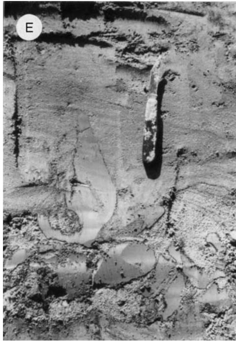
Figure 7.20: Schematic vertical section showing Holocene sediments (nonliquefiable cap and underlying Wisconsinan age source sand that liquefied). Exposure is in a ditch in the meizoseismal region of the 1811–1812 New Madrid earthquakes. Earthquake-induced intrusions cut section at many places. (A) Schematic diagram of stratigraphic relations and liquefaction-induced features (numbered 1–5). Feature 1, dikes of medium-grained sand that cut cap and source sand; features 2 and 3, intruded dikes and sills of massive, clean, medium-grained sand; feature 4, dike and flame structures of medium-grained sand containing and large clasts from bed G; feature 5, dikes of medium-grained sand, truncated unconformably; feature 6, pseudonodules collapsed in bed D. (B) Photograph of beds A–D showing sand intrusion (feature 3). Knife is 12-cm long (B–E). (C) Photograph of dikes (feature 1) cutting source (bed A) and bed B. (D) Photograph of plan view of bed B showing intrusion structures caused by feature 1; the plan view is in the area of the knife that is oriented vertically in part (B). (E) Photograph of part of feature 4, showing clay clasts in sand matrix intruded into bed H.
