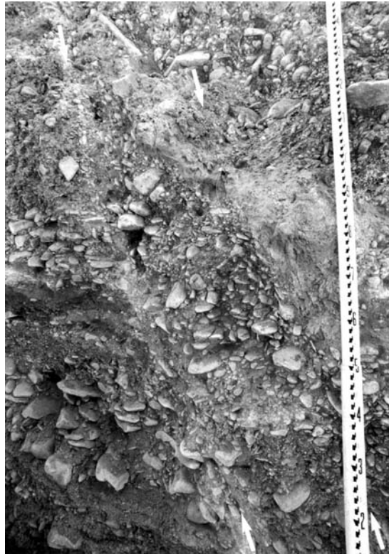
Figure 2A.34: Close-up photograph of two parallel normal fault strands (between arrows) in gravelly late Pleistocene deltaic deposits, East Bear Lake fault, Utah. Numbers on rod are 10 cm apart. Note anomalous parallel clast fabric and slight discoloration of gravel along the fault strands.
