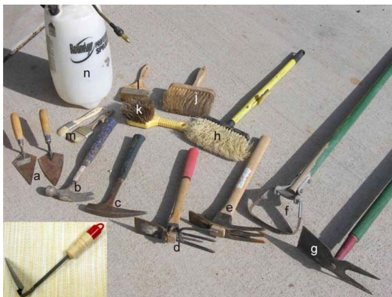
Figure 2A.32: Cleaning tools commonly used in North America: (a) masonry trowels; (b) claw hammer, claws are used for plucking; (c) geologist's hammer; (d) lightweight gardening mattock; (e) heavier gardening mattock; (f) stirrup hoe; (g) weeding hoe; (h) broom; (j) drywall brush; (k) scrub brush; (l, m) paint brushes; (n) portable water sprayer. Inset: a Nishiri gama hoe from Japan, favored by many professionals.
