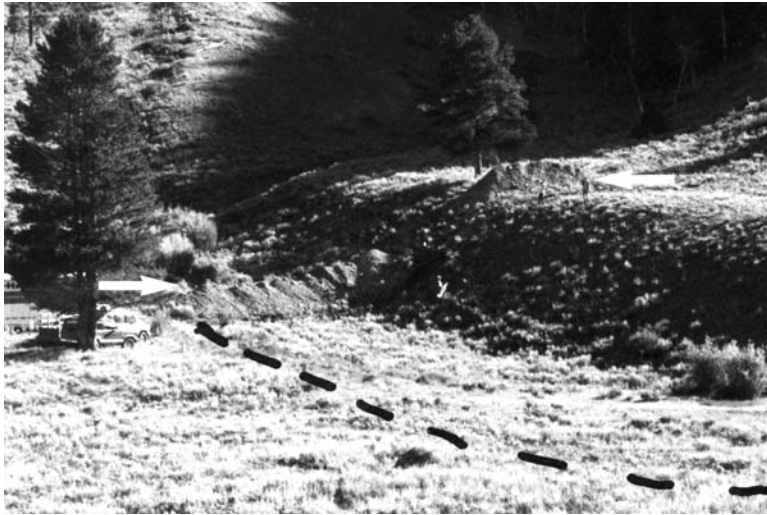
Figure 2A.20: Photograph showing the orientation and placement of a trench (between arrows) across an 8 m-high normal fault scarp (in shadow). The trench completely traverses the scarp, from well onto the upthrown block, to well onto the downthrown block, thus exposing pre-faulting strata on both the footwall and (if the trench is deep enough) on the hanging wall. A zone 10 m wide at the foot of the scarp has been back-tilted toward the scarp; the hinge line of tilting is shown by a dashed line. Grey's River fault, Wyoming (Jones, 1995).
