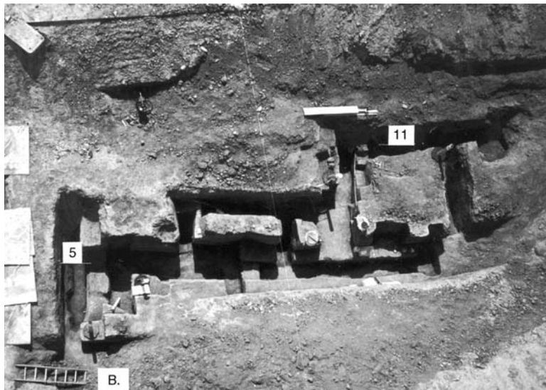
Figure 6.45: Vertical photograph of trenches 5–11 at the Rose Canyon site. Trenches 5 and 11 are labeled for reference. Note aluminum hydraulic shore (light-colored object above and left of “11”) for scale; its total length is 2.8 m. North is to lower right corner. Note numerous benches within excavation. For further details, see Lindvall and Rockwell (1995).
