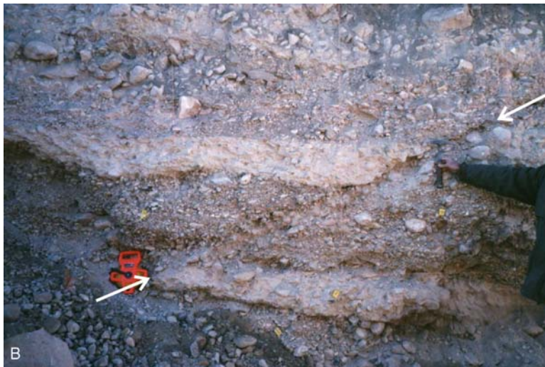
Figure 2A.14: GPR defines a thrust fault target on an alluvial fan. (A) GPR profile across the fault scarp on the alluvial fan; (B) Photograph of the thrust fault in the trench wall. The outline of the trench is shown. The thrust fault is well defined by a reflector dipping to the west (left), which is well defined below the depth of the trench, but poorly defined in the trench; From Anderson et al. (2003).
