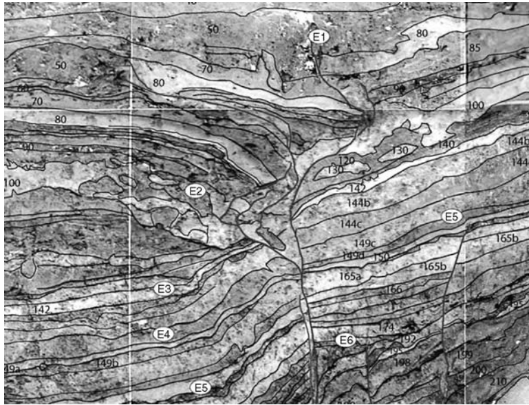
Figure 6.39: Photomosaic of the south wall of trench T4, cut 3, at the Hog Lake trench site, showing evidence for the latest five paleoearthquakes E1–E5; individual photos are 1 m 2 . Note the repeated section of unit 80 (uppermost light-toned bed) by event E1 (the most recent earthquake), which can only be resolved with strike slip. Penultimate earthquake E2 is only represented by liquefaction and disruption of unit 100, overlain by a bedded section. Earthquake E3 is represented by an angular unconformity and folding, as are earthquakes E4 and E5, but E5 is also represented by an upward termination on a secondary fault at far right. From Rockwell et al. (2004).
