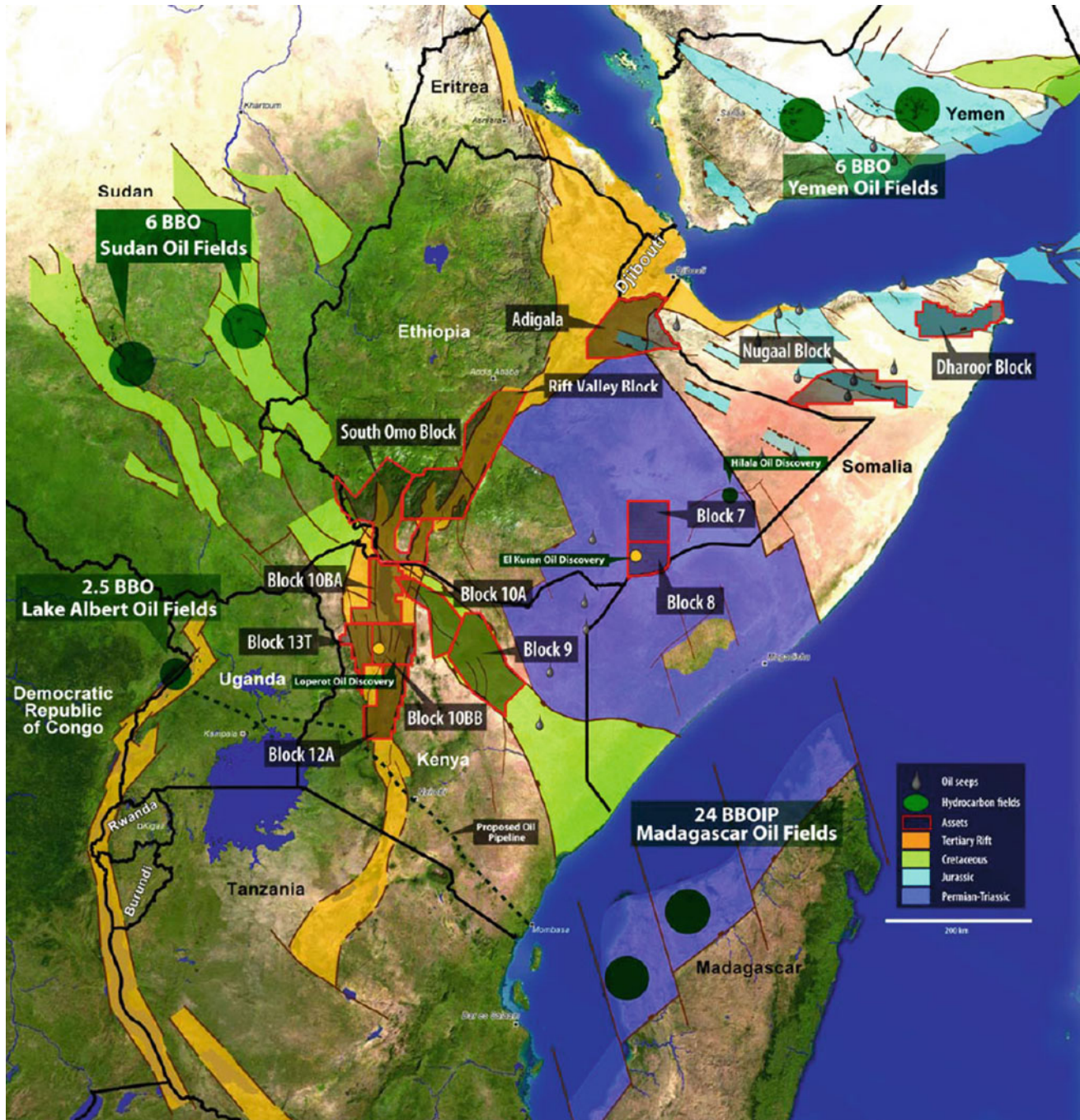
Fig. 4.3 Schematic map of East-Africa and southern Arabia (Yemen) showing the location of the various rifts as well as oil exploration and production blocks. Permian basins (Somalian plateau and Madagascar coasts), Jurassic WNW trending grabens of N Somalia and Yemen, NW to NNW trending cretaceous oil bearing grabens in Sudan, with its
