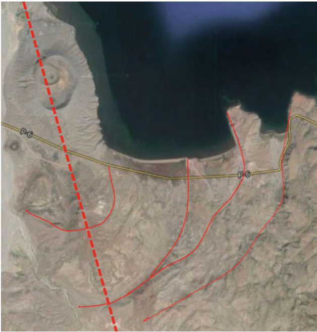
Fig. 7.13 The volcano-tectonic structures observed on the south and western shore of the Gulf of Zula, as seen from satellite image (USGS Earth Vision). A set of volcanic centres are aligned along a NNW (Red Sea) direction, with successive collapse structures developed from SE to NW, the most recent being two imbedded hyaloclastite cones along the western coast of the gulf
