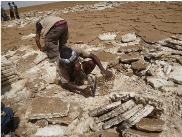
Fig. 7.9 The salt slates are then cut in regular rectangles, cleaned by peeling the clayed surfaces, and piled with the right shape for commercial use (Photos Varet 2015)
