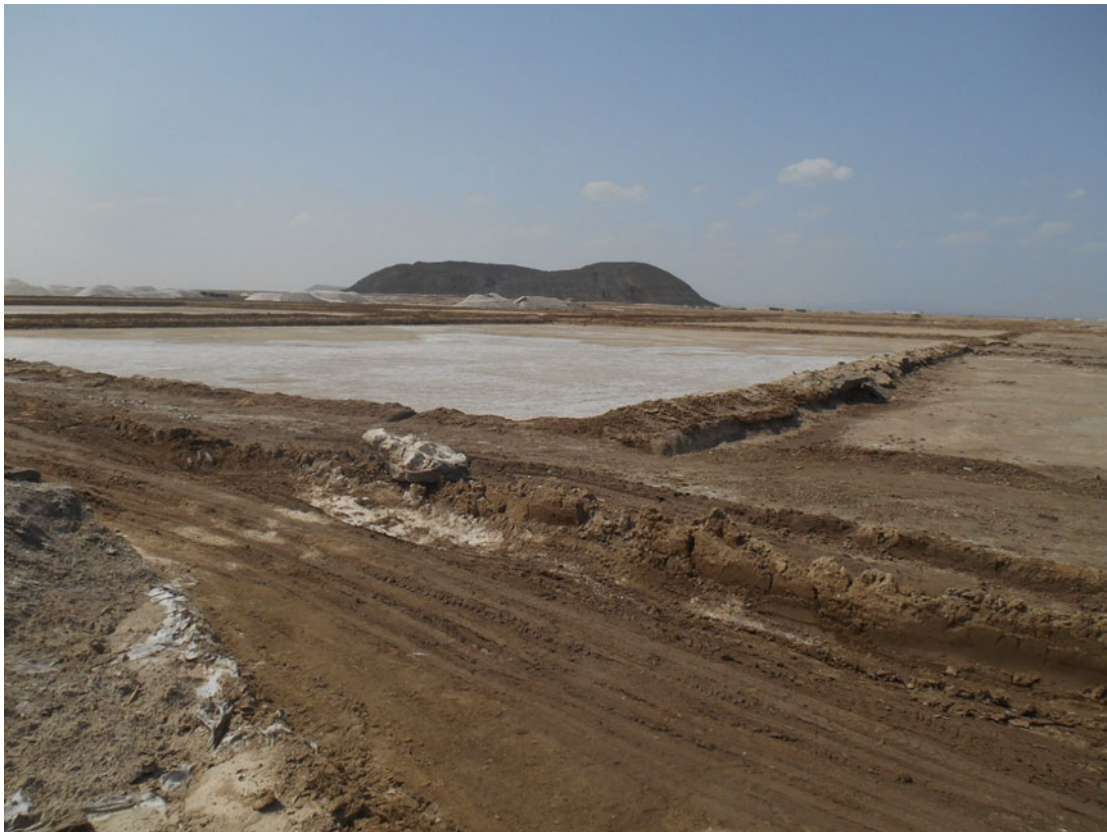
Fig. 7.32 Salt evaporation ponds built around Lake Afrera. The saline water of the lake is pumped up into these ponds where the salt precipitates. In the background is a subaqueous hyaloclastite cone ( Photo Varet 2015)
