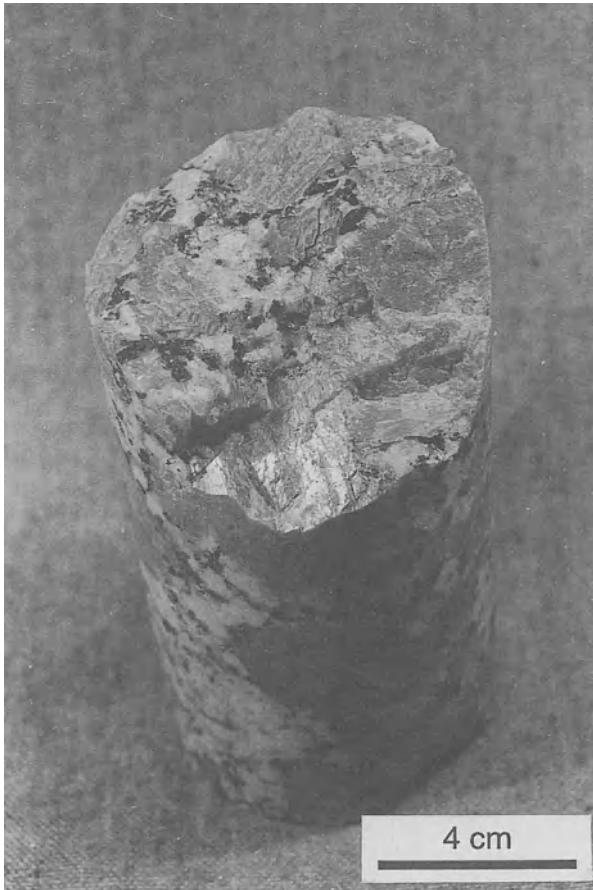
Figure 4. Photograph of a core-drill from the Soutz granite containing feldspar phenocrysts with well visible cleavages.
