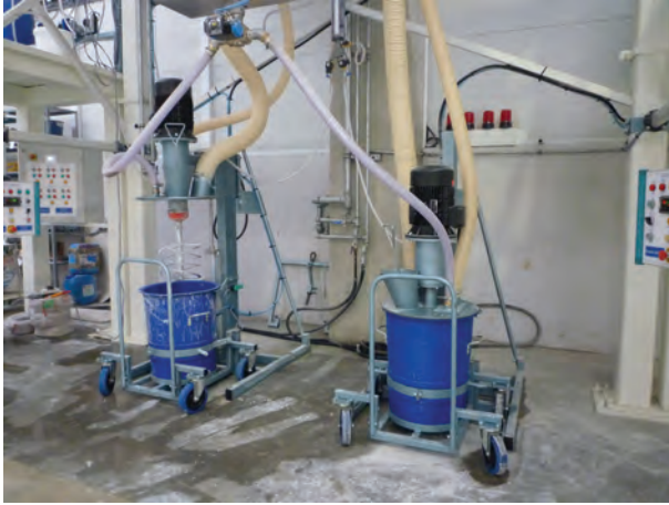
Figure 4.1 Typical GRC 125 Combination high shear batch mixers. (Courtesy of L. White.)
