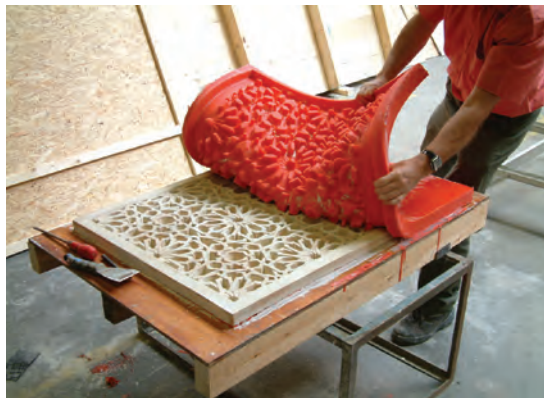
Figure 4.9 Polyurethane rubber mould being stripped off. (Courtesy of the iGRCA.)
