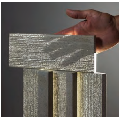
Figure 4.7 Section through light-transmitting glass fibre concrete [38].
