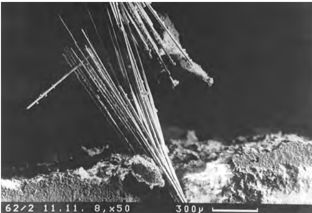
Figure 5.4 Fracture of a strand of fibres crossing a crack at an angle during a test within a SEM. Note the broken fibres at the sides, where the edges of the matrix ‘cut’ into the fibres. A small number of fibres in the interior of the strand still cross the crack and carry load [46].
