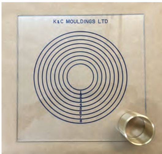
Figure 6.1 Basic arrangement of the (mini) slump test for fresh slurry [51].
