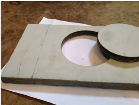
Figure 4.15 A GRC sheet with a very precisely cut hole using a laser beam. (After N. Charlesworth.)
