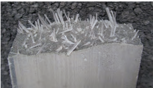
Figure 5.3 Flexural test fracture surface – premix GRC. Almost all of the fibres remained bundled in strands.
