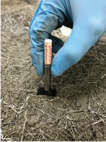
Figure 4.6 A thickness gauge being used to measure the thickness of a GRC sheet during production. (Courtesy of L. White.)
