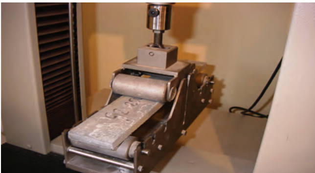
Figure 6.5 Typical test jig for the standard bending test.
