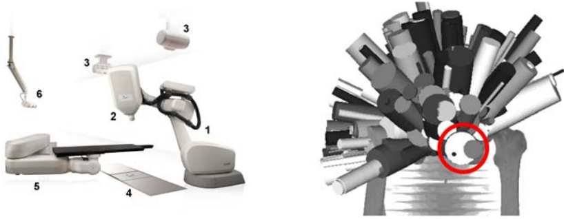
Fig. 1. The robotic CyberKnife system by Accuray Inc. The system consists of a robotic arm (1), linear accelerator (2), X-ray sources (3) and orientation, diameter, and weight of the beams cameras (4), a robotized patient couch (5), and an optical tracking system (6). (Image courtesy of Accuray Inc.) Fig. 2. An illustration of the set of treatment arm beams used to irradiate a prostate tumor. The beams are shown in various orientations and diameters, with a red circle highlighting a specific beam. The beams inside the circle start in the same node, but have different diameter and orientation.
