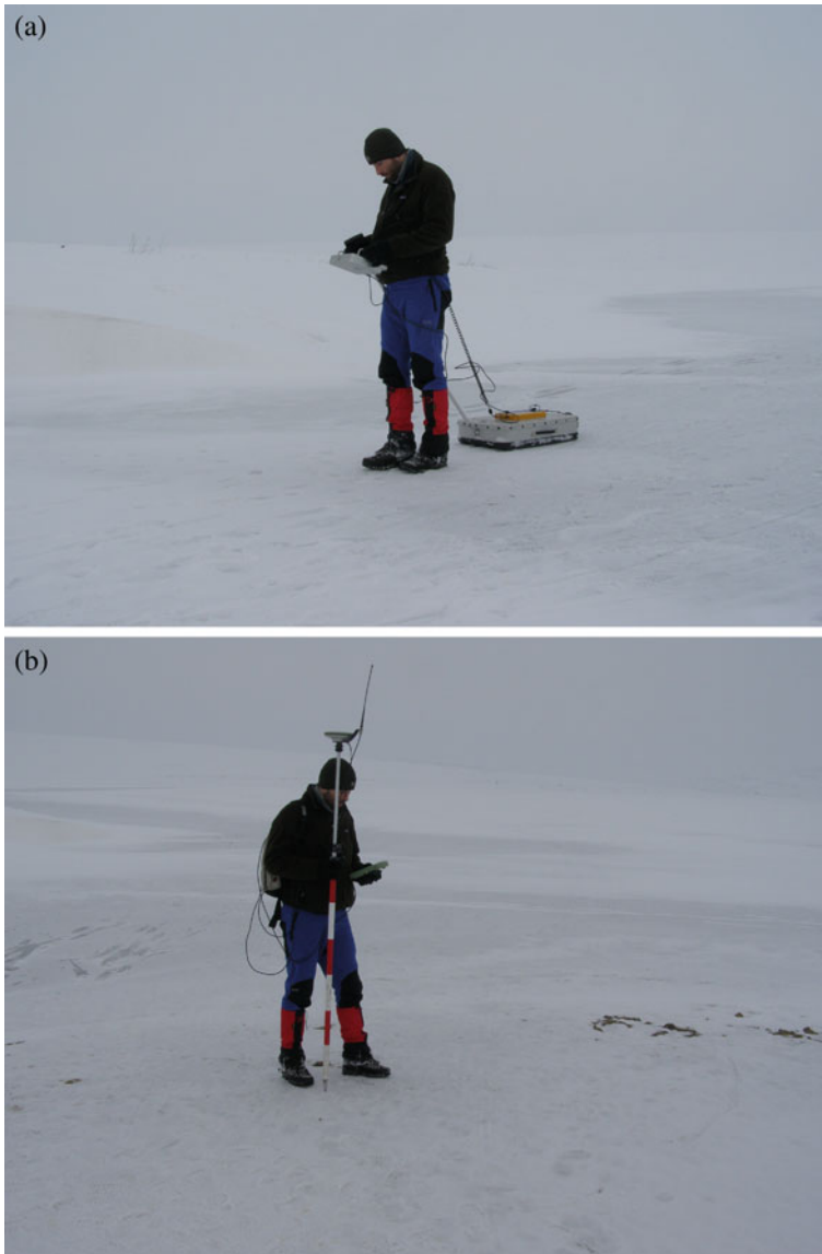
Fig. 11.8 a GPR surveys with 250 MHz shielded antenna; b GPS used to georeference GPR profiles
