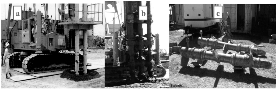
Figure 6.17 (a) CDM machine with two augers (after Raito Kogyo, 2006), (b) CDM machine with three augers (after Keller, 2005), (c) two augers which have been parted-off (after Balvac, 2008).
