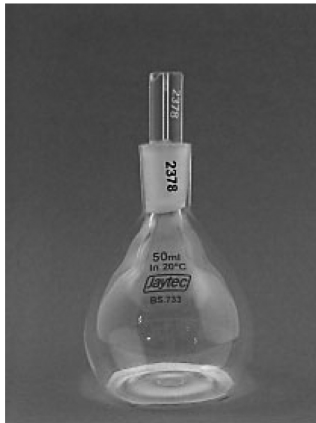
Figure 3.10 Density bottle used for measuring soil G_s in the laboratory (courtesy www.jaytecglass.co.uk ).
