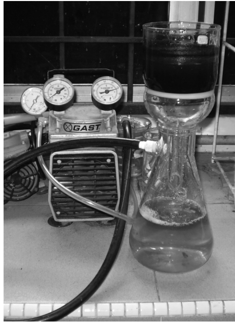
Figure 8.2 Motorized extraction for preparation of peat pore fluid.
