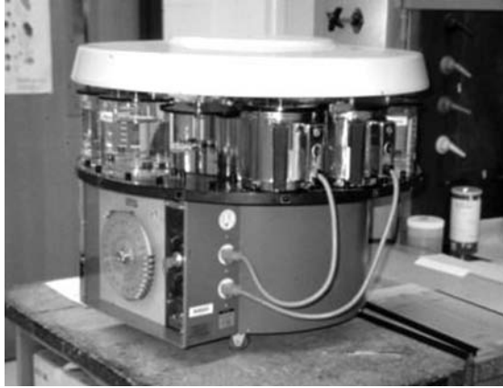
Figure 36.3 A basic tissue processor can speed up the dehydration, clearing, and infiltration steps and provide consistent results. (Photo by E.C. Peters.)
