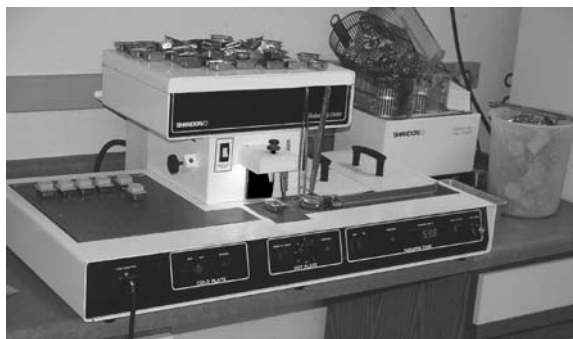
Figure 36.4 Basic embedding center consists of molten paraffin dispenser (top center), paraffin bath for tissues (back right), mold warming tray (front right), forceps warmers (front center right), hot plate (front center), and cold plate for hardening the blocks (left). (Photo by Jeffrey Greenberg, U.S. EPA, Atlantic Ecology Division.)
