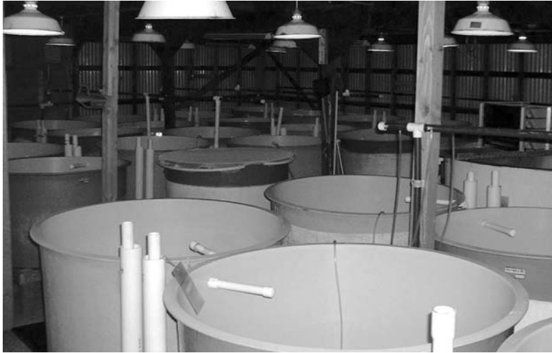
Figure 5.2 Picture shows an array of 1.3-m-diameter (500 l) fiberglass tanks. Total array is 32 tanks. Note the air supply lines, drain stand pipes, spray bars for water delivery (inside the tanks), overhead lighting, and the tank with mesh cover.
