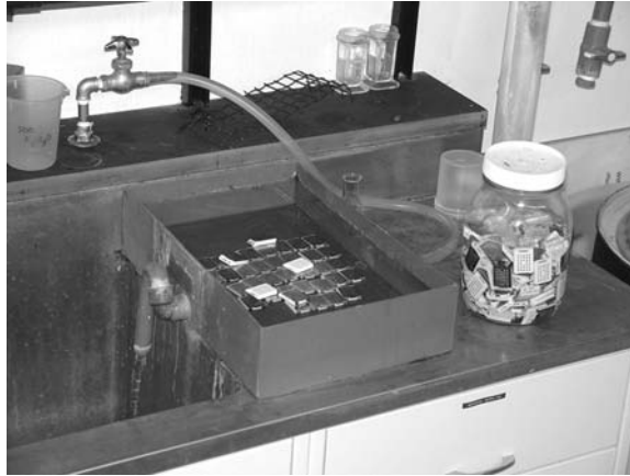
Figure 36.2 Self-siphoning water bath. Continuous filling and draining with tap water thoroughly rinses decalcified tissues (here in cassettes) for 24 h. (Photo by Jeffrey Greenberg, U.S. EPA, Atlantic Ecology Division.)
