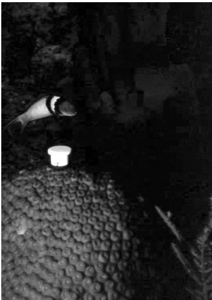
Figure 29.2 Passive dosimeter mounted underwater.
