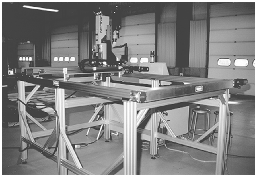
FIGURE 3.9 Fully automated Z-Fiber insertion robot.
