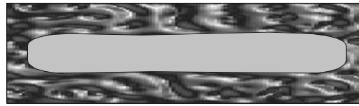
Bulk Degradation (section)
