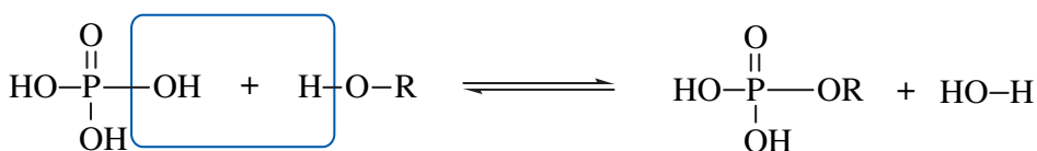
Figure 11.53 Formation of a Phosphate Ester
