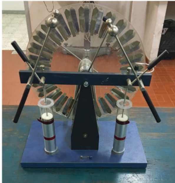
Fig. 11.1. Wimshurst machine used in a teaching laboratory in the Physics Department in the Federal University of Santa Maria
