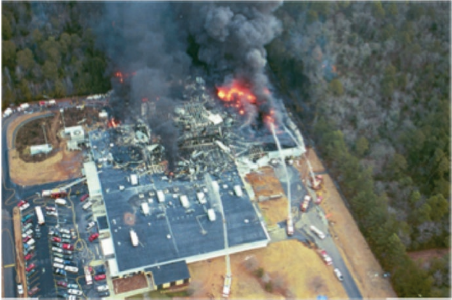
Fig. 12.3 Picture taken from the site of a factory after an explosion assigned to polyethylene dust. Reprinted with permission from Ref. 38
