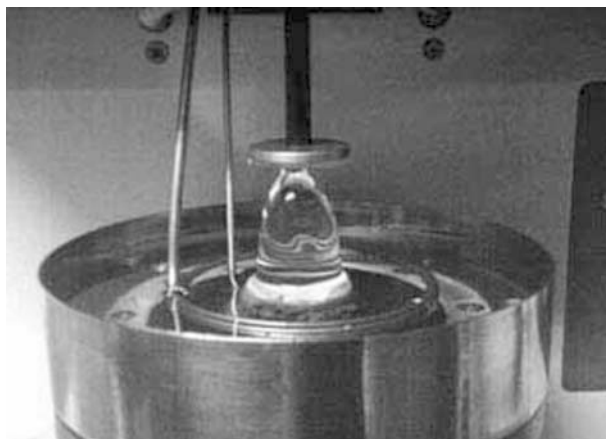
Fig. 8 Photograph of the erosion of a gel with C = 2.0\text{wt}\% took place after 400 min. identified in the sample chamber
