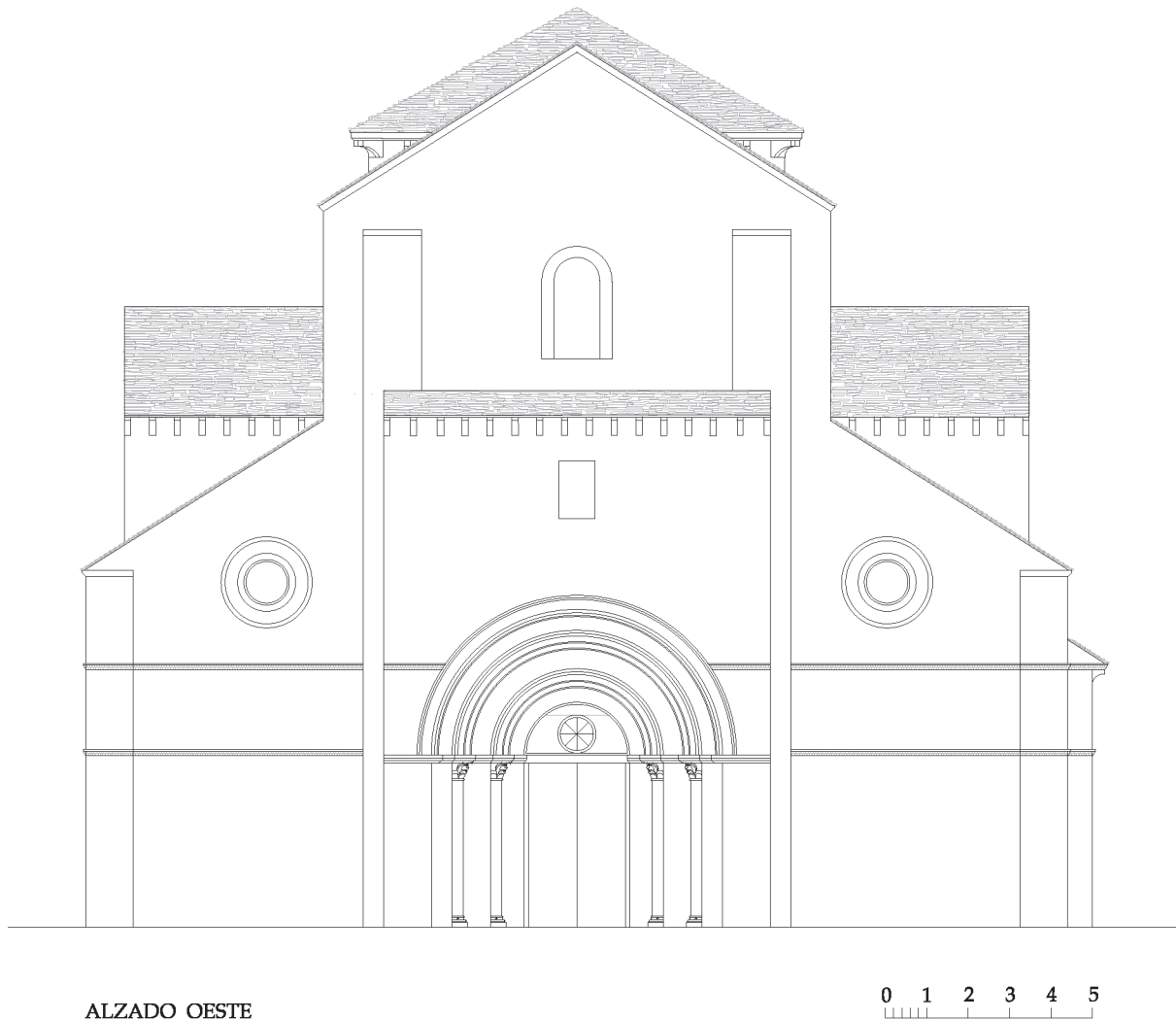
Fig. 6. Graphic reconstruction of Jaca Cathedral: west façade elevation around 1100 (proposal by author, drawn by Marina MARTÍNEZ DE AGUIRRE from plans designed by Ricardo MARCO, Jesús MARCO, and Javier IBARGÜEN)
