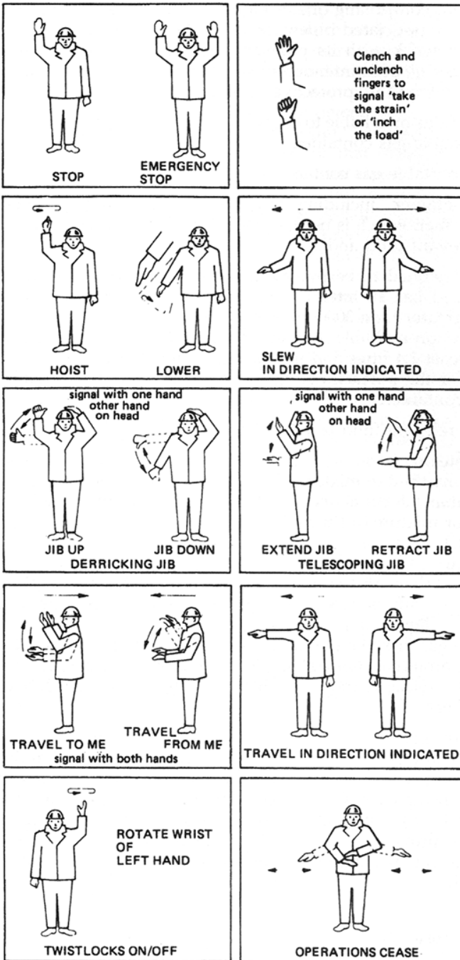
Figure 3.19 Crane signals. (BS 7121)
