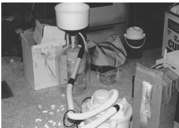
Figure 9.14 Vacuum filtration with shop vac as vacuum source.
