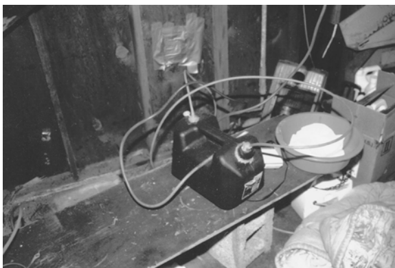
Figure 9.17 Hydrogen chloride gas generator.
