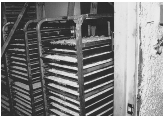
Figure 9.15 Vapor explosion fire damage.
