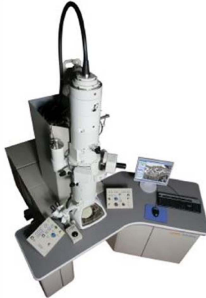
Figure 1.2 Transmission electron microscope. This is a microscope in which the image is formed by electrons transmitted through the specimen.
