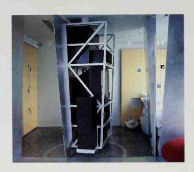
Attached to one of the aluminum panels, the media center pivots to face either the bed or the conversation area.
