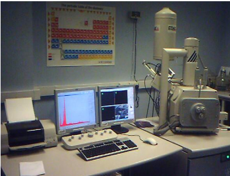
Figure 9.5 The FEI Quanta 600 scanning electron microscope is one of the devices used to assess a variety of S&T factors from biomass and fossil fuel samples. Source: Author.
