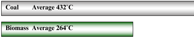
Figure 6.4 South African bituminous coal (Kleinkopje) and biomass average ignition temperature (dry matter). Source: Author.
