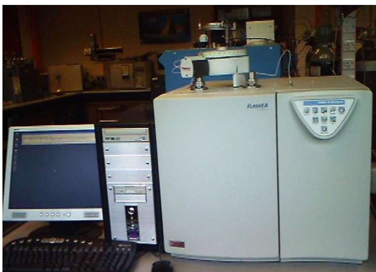
Figure 9.3 Thermo Electron Flash EA 1112 series 3. Source: Author.
