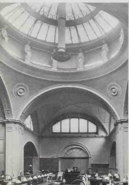
339, 340 Soane: above, the breakfast parlour in his house in London (1812); below, the Consols Office of the Bank of England (1794). The arches are segmental, not round. The plasterwork has a flat Grecian delicacy. Above, light enters indirectly and gleams in convex mirrors. Below, the flat surfaces are piquantly contrasted with the fully modelled caryatids in the cupola
