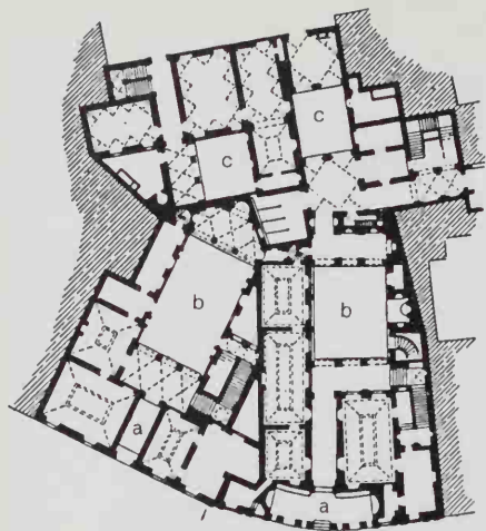
211 Plan of the palaces in Rome designed by Peruzzi for Angelo (left) and Pietro Massimi, 1535. Opening off a curving road, each has a vestibule (a), grand cortile (b) and minor court (c)
