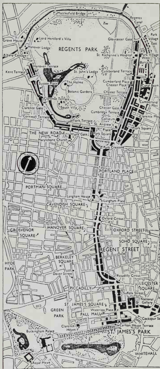
328 John Nash's plan for London (1812–27) – marked in black – linking Regent's Park to St James's Park, had to be laid across the existing town. It is therefore more irregular than, say, Nancy or Bath. Also, the new cult of the Picturesque explains a quite deliberate informality in the design of the parks themselves and the terraces
