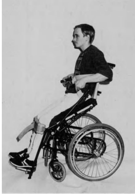
Fig. 11. The Levo active wheelchair in half up position
