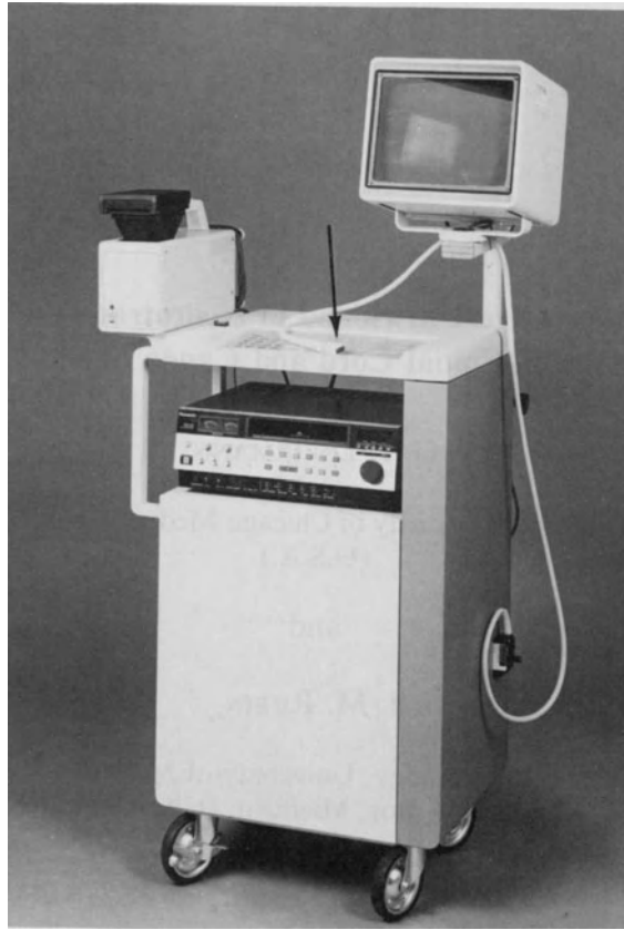
Fig. 1. Real-time ultrasound scanner designed for intraoperative use. Scanhead (arrow) is resting atop the pressure-sensitive control panel; videorecorder is seen below. Polaroid camera is attached to scanner on left; videoscreen is on right. (Codman and Shurtleff, Inc., Randolph, MA 02368, U.S.A.)
