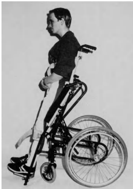
Fig. 12. The Levo active wheelchair in standing position
