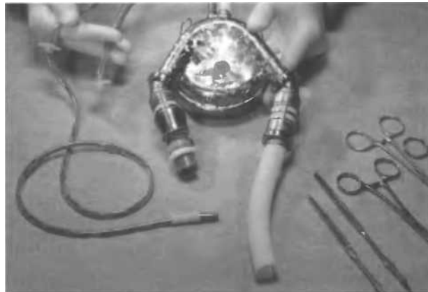
Figure 5 The TCI HeartMate VE LVAD. The left ventricular outflow attachment is on the left and the aortic inflow graft is on the right
