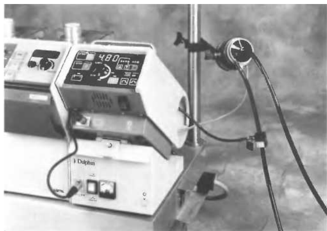
Figure 2 The Sarns centrifugal blood pump. The spinning pump head continuously drains and returns blood with non-pulsatile flow
