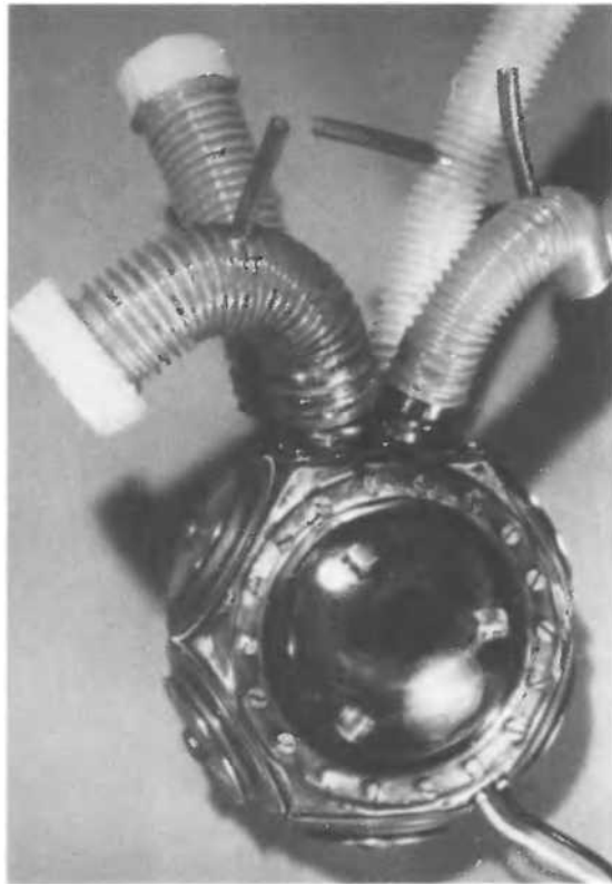
Figure 5 Five solenoids are arranged in a rosette. When energized they compress a hydraulic fluid that is within the housing. On the top of the artificial heart one sees the atria, the pulmonary artery, and the aorta. These vessels are made of corrugated polyurethane so they can bent without kinking
