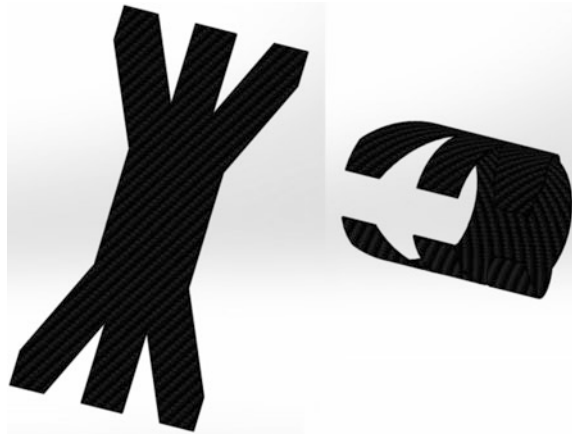
Fig. 12 Example of composite hand: after the memory step ( left ) and in the final configuration ( right )
