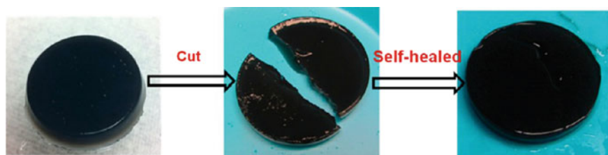
Fig. 10 Graphene-incorporated PAM hydrogel exhibiting self-healing property [85]. Copyright 2013. Reprinted with the permission from the American Chemical Society
