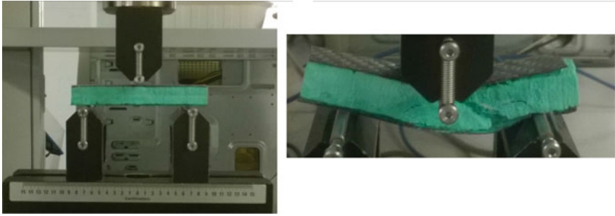
Fig. 17 Bending test ( left ) and failure of SMC sandwiches with epoxy foam core ( right ) [3]. Copyright 2016. Reproduced with permission from Elsevier
