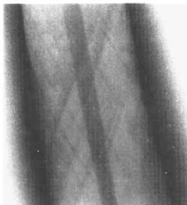
Figure 37 Electron micrographs of self-assembled fibres. (a) Porphyrine-fibres with a diameter of 6 nm. (b) N -octyl- D -mannonamide multilayered fibre, negatively stained with phosphotungstate, the central dark hole has a diameter of 50 nm. (a) and (b) were obtained from aqueous solution [424].
