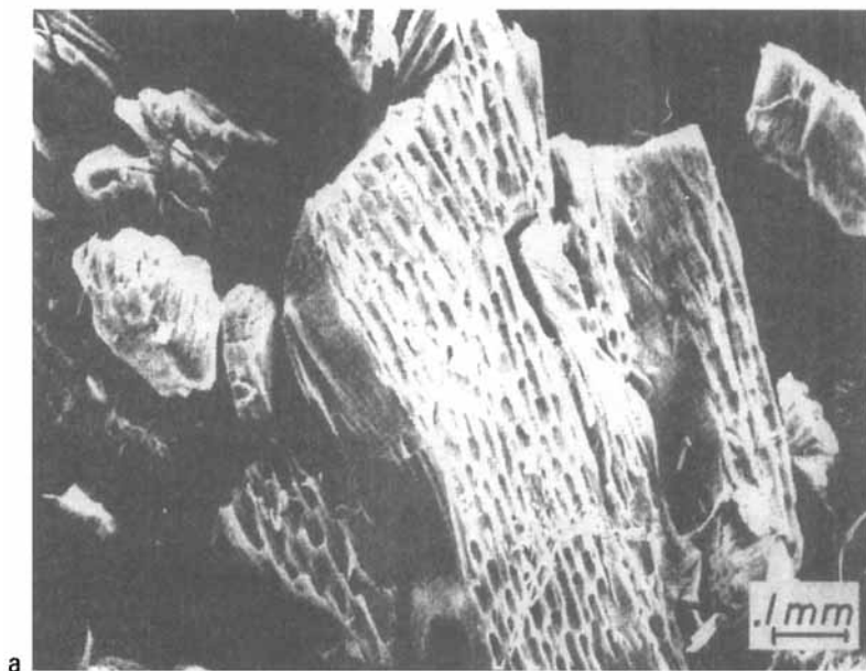
Figure 17 (a) Topochemically polymerized poly(oxymethylene) exhibiting cylindrical voids. Reproduced from [186,187]. © 1981 John Wiley & Sons Inc., with permission.
