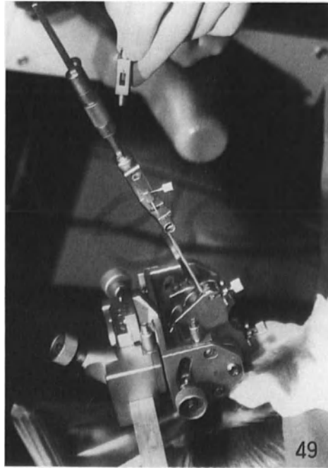
Fig. 48. The Riechert-Mundinger apparatus for CT guided stereotaxy (by courtesy of Prof. Mundinger)
