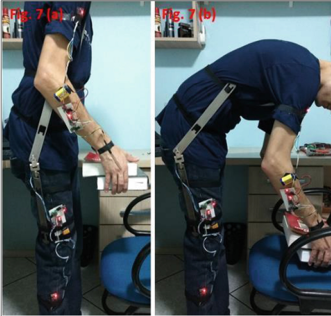
Fig. 7. Ergonomic vestment prototype simulation. Sensors devices mounted on the user to execute the tasks and to send the sign (angles) via Arduino to the computer database. (a) Safety position or green condition. (b) Alert position or yellow condition.
