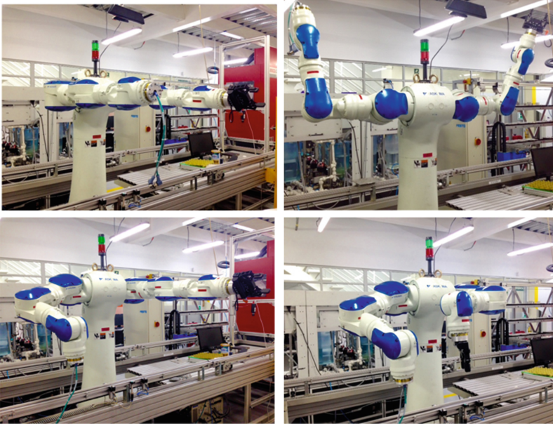
Fig. 7. Poses defined in the SDRF file from Motoman MoveIt—config file
