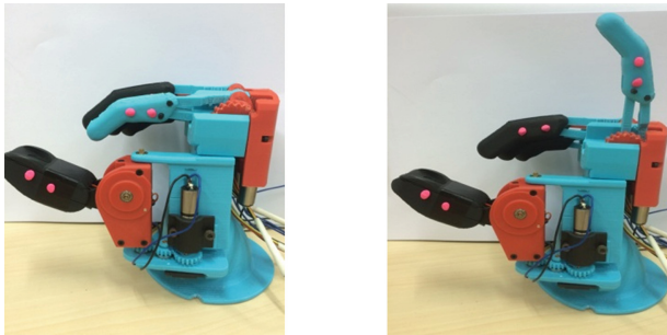
Fig. 11. Flexion and extension velocity measurement for the index finger.
