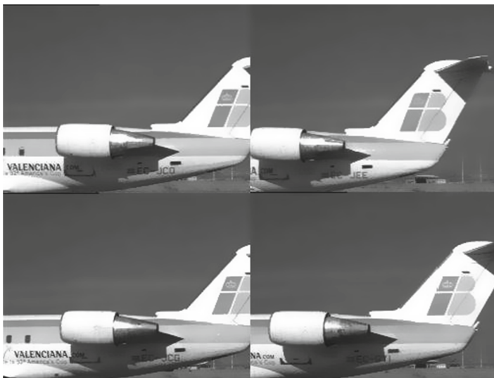
Fig. 6. Problems with shadows over the aircraft tail number.
