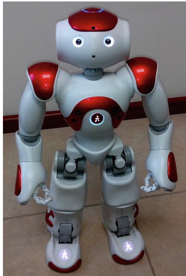
Fig. 1. The Nao humanoid robot from the Aldebaran Company.
