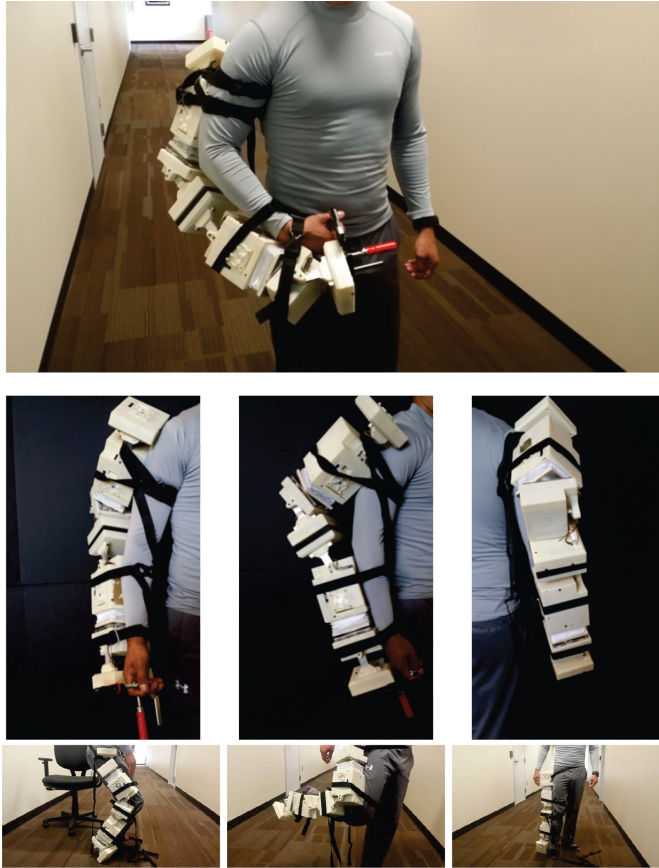
Fig. 4. Two ModRED II modules (in a chain-type configuration) have been attached to the upper and lower limbs of the human body with the purpose of analyzing their workspace and performance when working with different muscles and joints.
