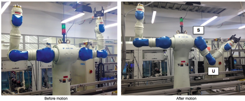
Fig. 8. Joints motion test. The MoveIt!’s API allows to send joint commands to the robot. The figure shows the robot when moving joints L and U. Left image shows the starting position, and right image the final position.
