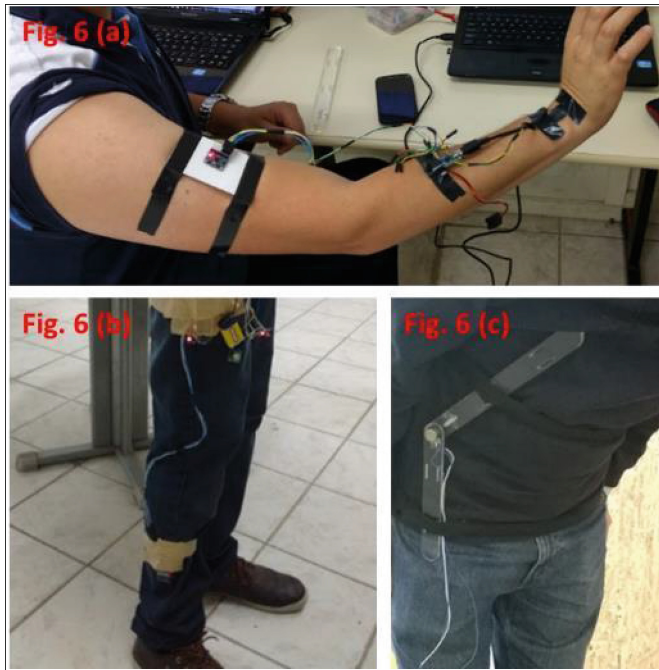
Fig. 6. Ergonomic vestment prototype real system. (a) Arm, forearm and wrist subsystem, related to the Fig. 5(a). (b) Legs subsystem, related to the Fig. 5(b). (c) Trunk subsystem, related to the Fig. 5(b).
