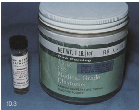
Fig. 10.3. RTV ("Room Temperature Vulcanizing") silicone elastomer from Dow Corning, shown with its stannous octate catalyst. (This product is no longer marketed in the U.S.)
