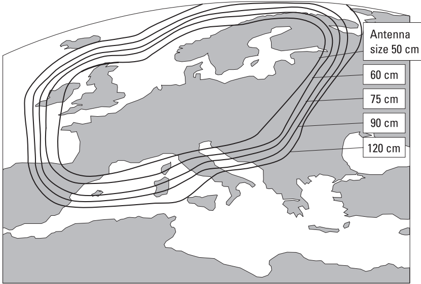
Figure 12.2 Typical footprint of a GEO TV satellite beam directed at Central Europe.
