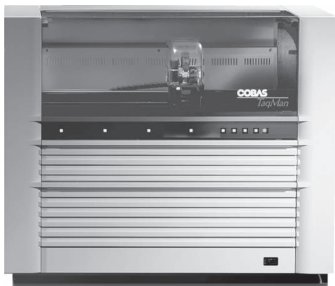
FIGURE 2-18 TaqMan instrument for performing PCR. Reprinted with permission from Roche Diagnostics Corp., Indianapolis, IN.
