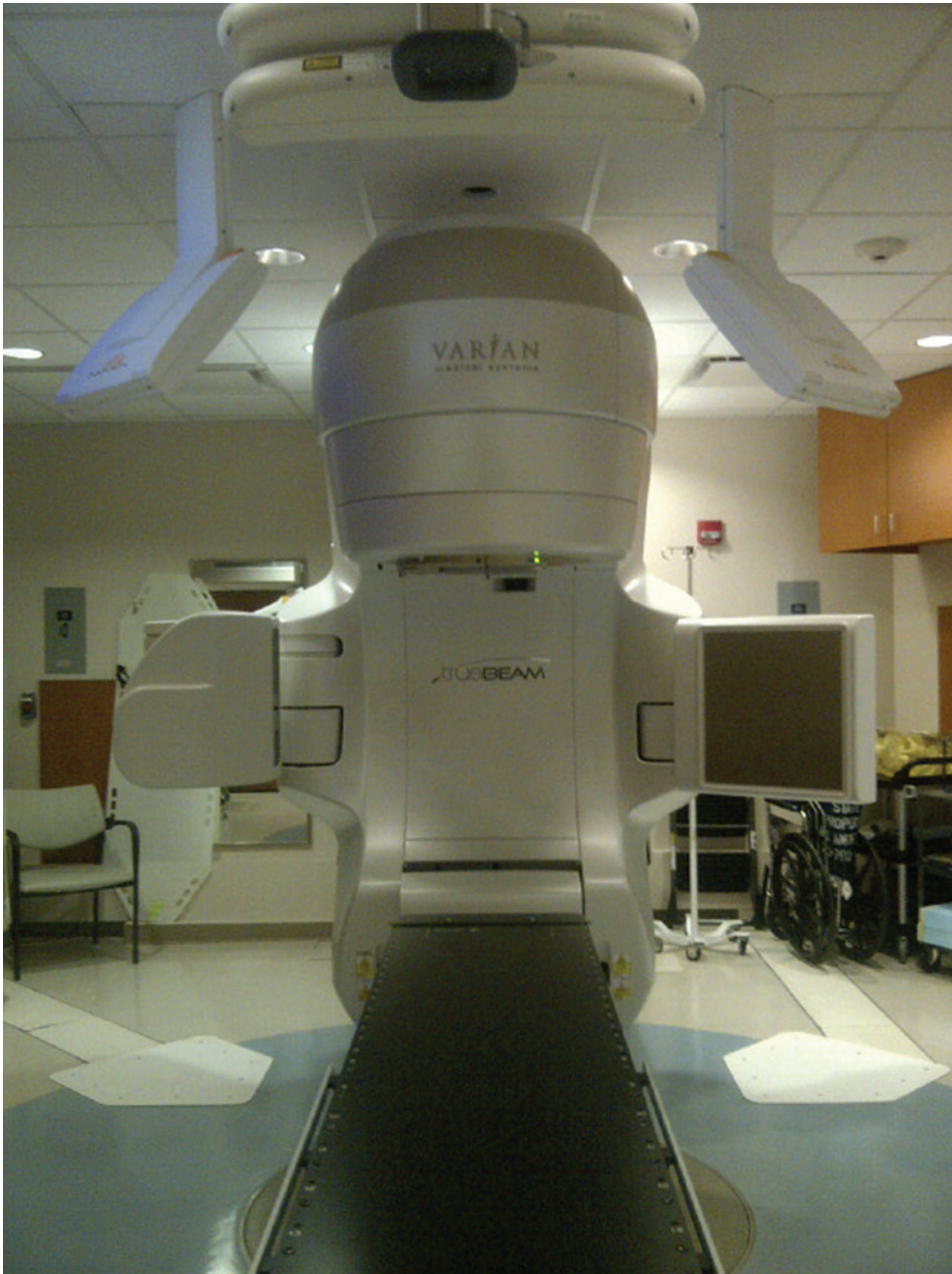
Figure 11.1 Varian TrueBeam™ linear accelerator with on-board kV imaging.
