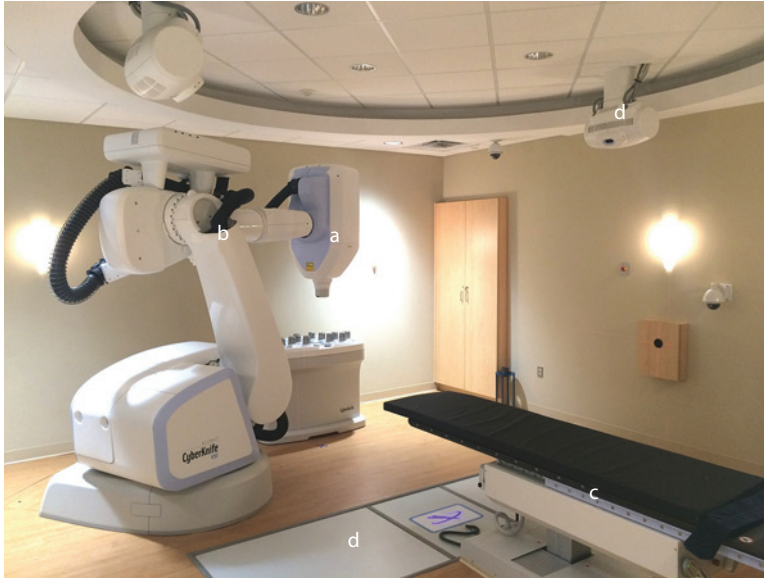
Figure 9.1 A typical CyberKnife® treatment room (Model G4). Components are labeled: (a) X-band linear accelerator, (b) six-jointed industrial robotic arm, (c) a standard treatment couch, and (d) x-ray tubes and detectors.
