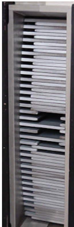
Figure 8.4 TomoTherapy® binary MLC are interleaved.
