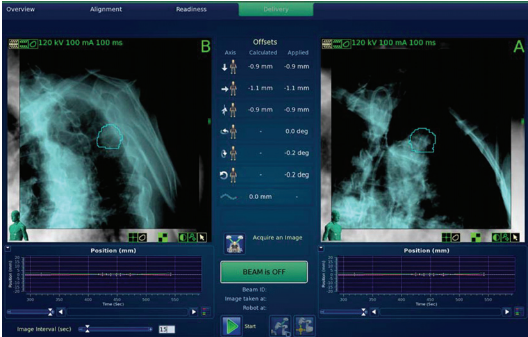
Figure 5.6 Screen capture of the tracking console software. The images show the acquired planar image in a blue overlay on top of the DRR. Images A and B each correspond to an orthogonal imager. The solid blue line outlines the tracking target volume and is positioned at the location the automatic tracking algorithm found the tumor.
