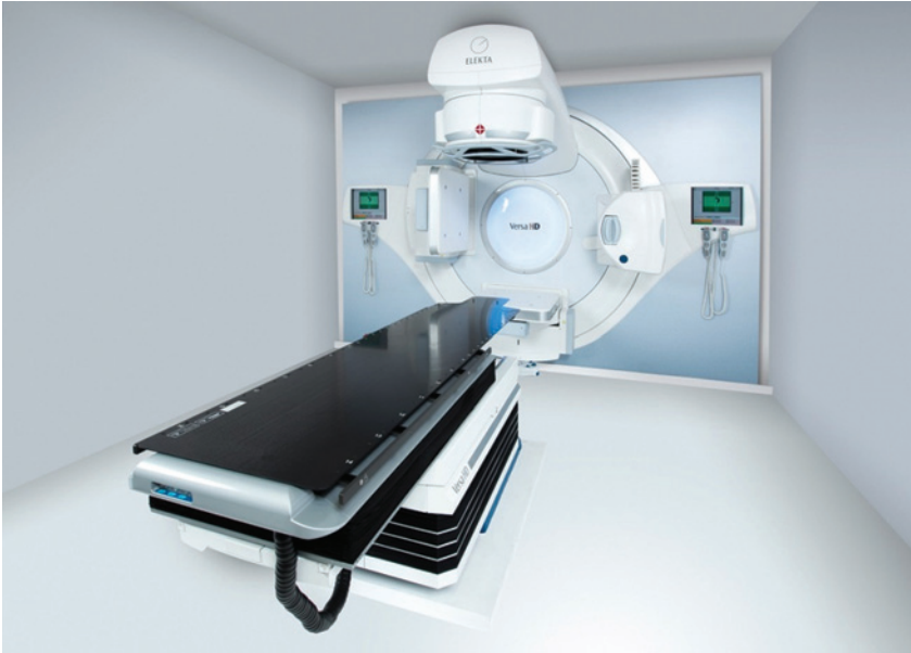
Figure 7.1 The Elekta Versa HD™ provides an array of IGRT tools, including two amorphous silicon panels for MV portal imaging, perpendicular kV imaging, and kV CBCT. 4D CBCT is possible to characterize patient motion, especially useful in the case of lung lesions.
