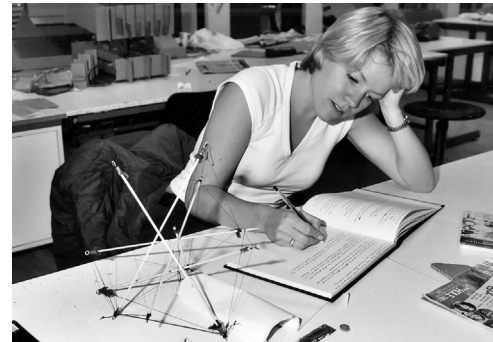
Figure 6-15 A model of a tensegrity structure.
