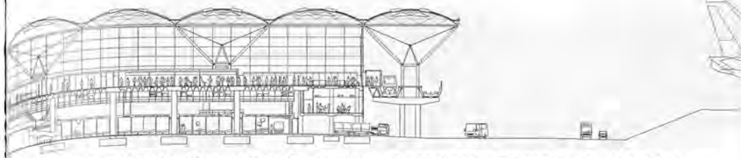
310 Foster Associates, Stansted Airport Terminal, 1991. North-south section. The roadway side is to the left, the runway side to the right.
