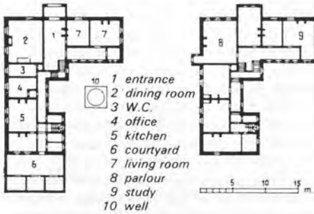
25, 26 Webb, Red House, Bexley Heath, Kent, 1859. View, and plans of ground and first floors.
