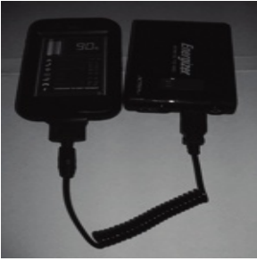
Figure 9.4 A small power pack (the size of a deck of cards), which adds several hours of operation to my netbook, while charging various other mobile devices when I am on the road (it is shown here charging my phone).
