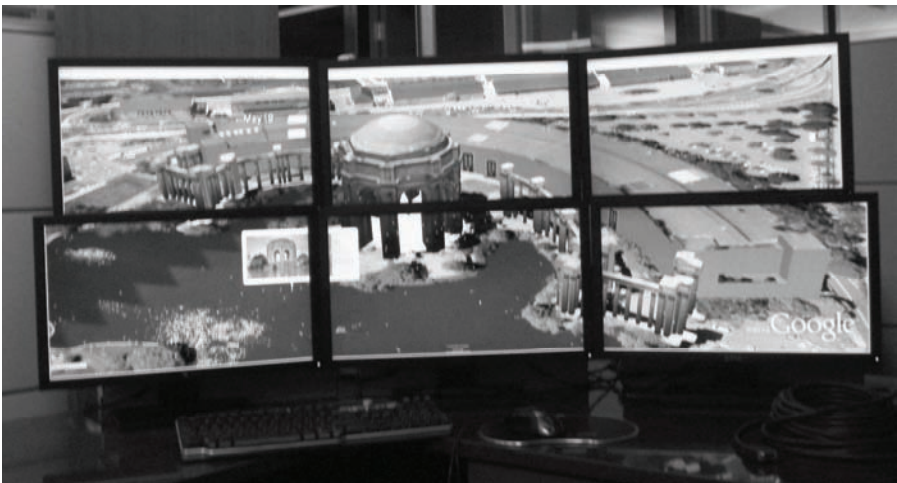
Figure 14.1 A small visualization cluster sharing the combined display area of six monitors to form a single large display.
