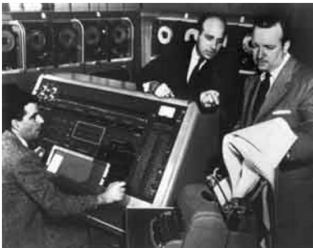
Figure 6.2. Photo of the room-sized UNIVAC 1 computer system that was introduced in the late 1950s. [8]
