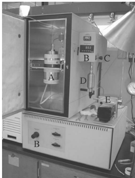
Figure C.2. Photograph of the supercritical fluid system used for nanoparticle synthesis. Shown is the 300-mL high-pressure reactor (A), with pressure/temperature controllers (B). The system is rated for safe operation at temperatures and pressures below 200°C and 10,000 psi, respectively. The vessel may be slowly vented, or exposed to a dynamic CO 2 flow, using a multistage restrictor valve (C), which provides a sensitive control over system depressurization, allowing for the collection of CO 2 -solvated species in the stainless steel collector (D). For deposition using the rapid expansion of the supercritical solution (RESS), nanoparticles were blown onto a TEM grid that was placed under the stopcock below D. Also shown is the cosolvent addition pump (E) used for the synthesis of aluminum oxide nanoparticles, capable of delivering liquids into the chamber against a back-pressure of \leq 5,000 psi.
