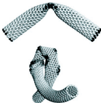
Figure 6.51. Illustration of the deformation modes of SWNTs, resulting in a high elasticity. This behavior is likely an artifact of in-plane flexibility of a graphene sheet, and facile rehybridization of carbon atoms from sp^2 to sp^3 geometries. Reproduced with permission from Ajayan, P. M. Chem. Rev. 1999 , 99, 1787. Copyright 1999 American Chemical Society.
