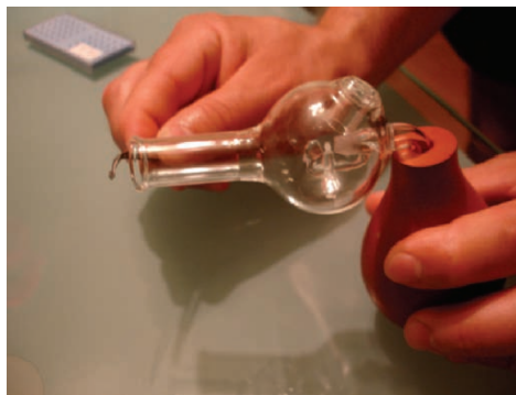
Figure 7.11. Photo of a glass aerosol delivery system used to spray solvent-suspended particulates onto a TEM grid.
