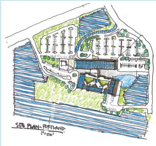
Figure 6.11 Site plan diagram. The site and rooftop is extensively covered with solar photovoltaic panels; a wastewater retention pond is used as a landscape feature. Source: SERA Architects
