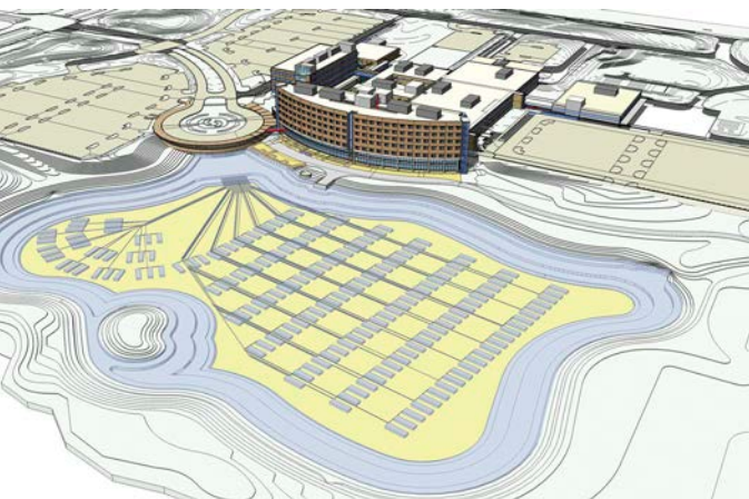
Figure 5.35 Diagram of lake, manifold room, and corridor from parking to hospital. Source: Image courtesy of Shepley Bulfinch
