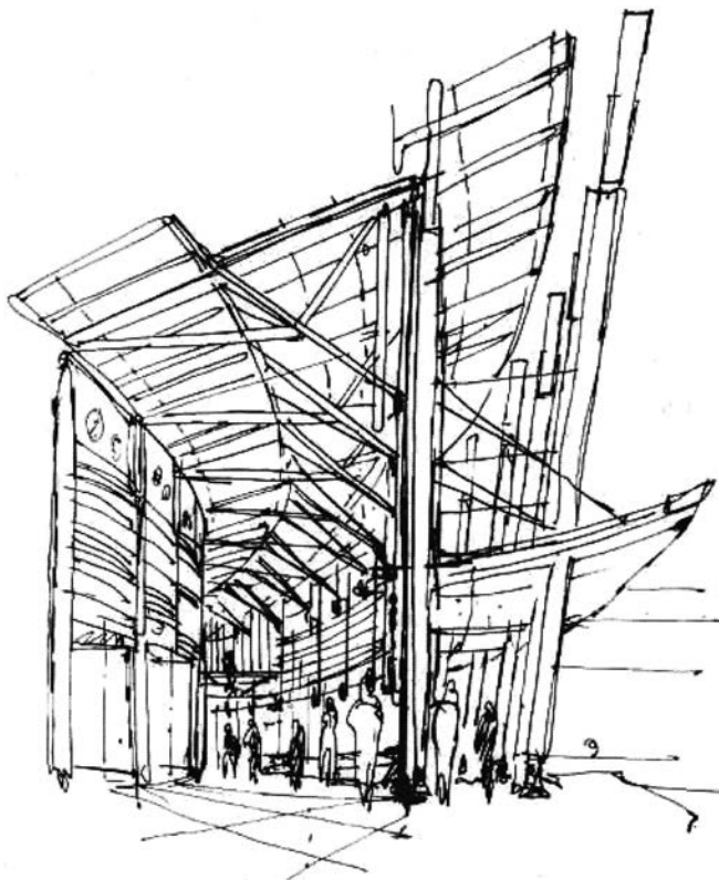
Figure 9.10 This conceptual sketch of the wood-structured main concourse at Thunder Bay illustrates the layering of the facade and structural elements. Source: Farrow Partnership
