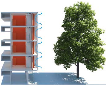
Figure 9.23 Facade section in summer. Source: Copyright © groupe-6
