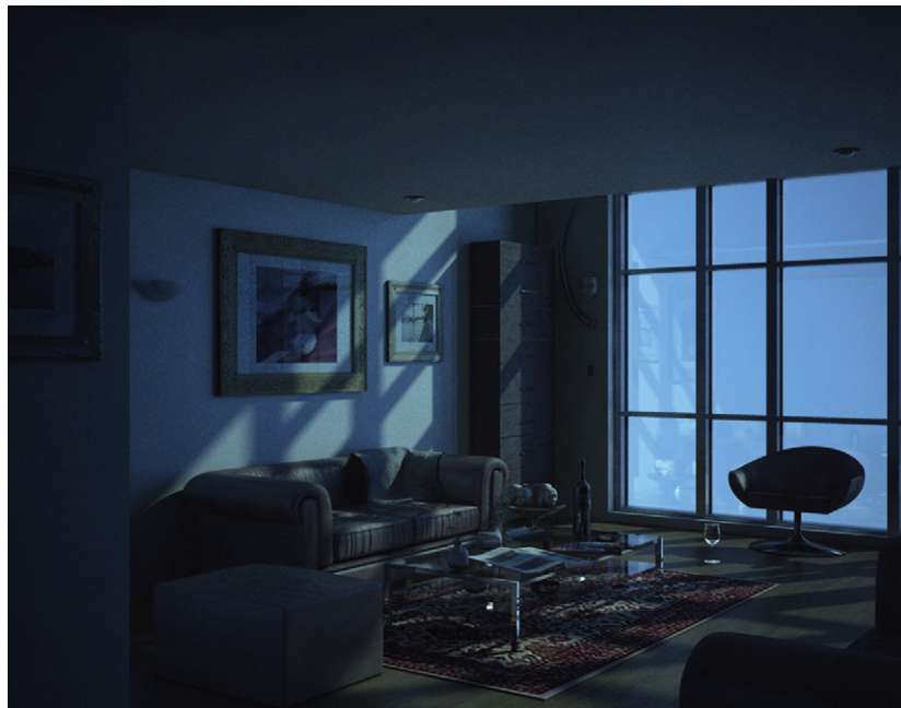
Light entering an interior space with a mr Sky Portal placed at the plane of the window glass, multiplier = 5.0
