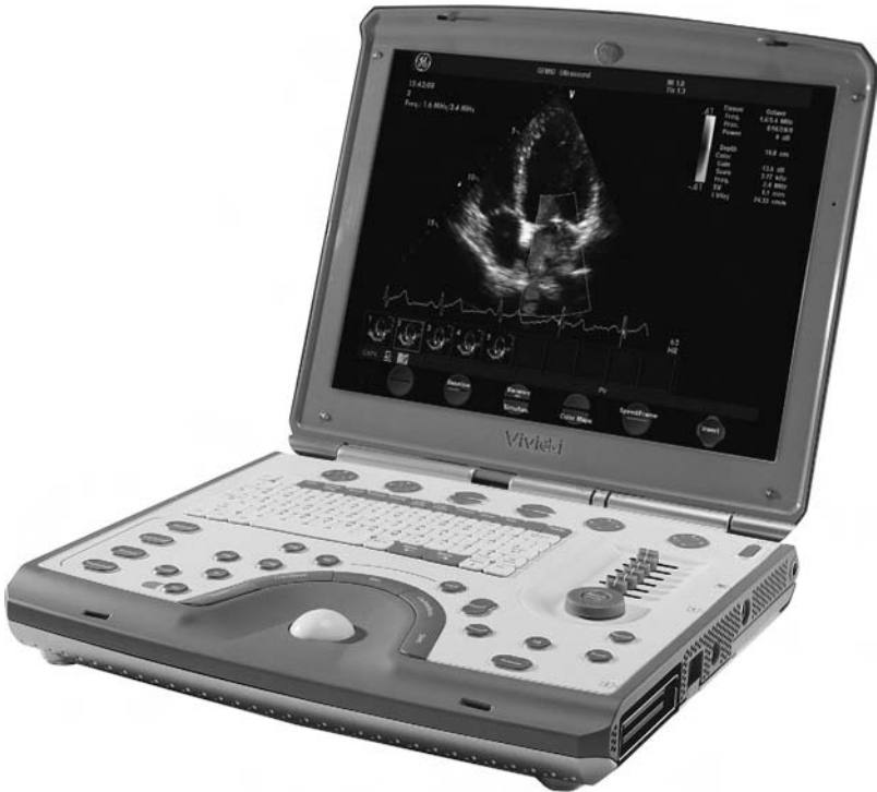
Fig. 7.6 The vivid- i , one of the new laptop-based portable echocardiographic systems. The performance and applications of these scanners can rival those of the large laboratory-based systems despite its compact size.
