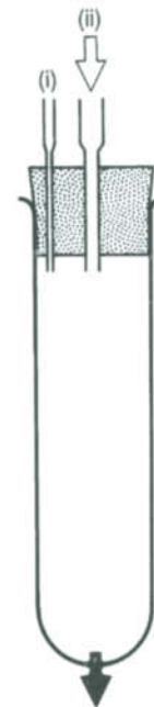
Figure 4.2. Apparatus for harvesting sucrose gradients (from Minor 1985).
