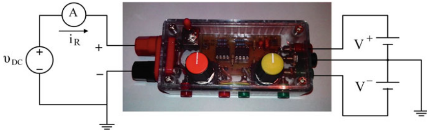
Fig. 11 The circuit for finding in analytical way the i-v characteristic of the nonlinear resistor of the Chua’s oscillator circuit
