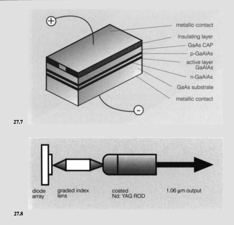
Fig. 27.7. Composition of single-stripe GaAlAs laser diode
