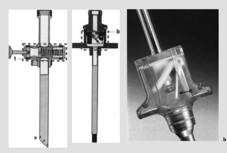
**Fig. 2.13a, b.** The types of valves used for cannulae. **a** On the *left* is a 10-mm cannula with a trumpet valve (*t*). On the *right* is the
