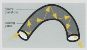
**Fig. 2.7.** Light passing through a glass fibre. On account of the lower diffraction index of the coating glass, the light is totally reflected
