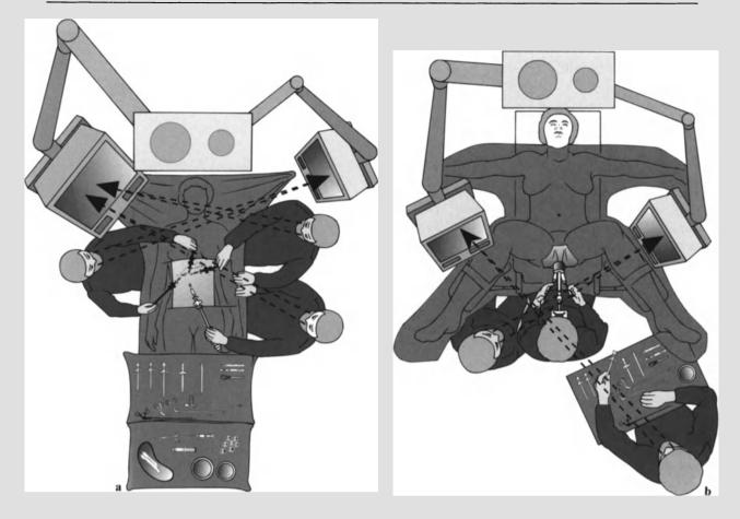
**Fig. 5.2 a, b.** The ideal method of positioning two monitors. The monitors are mounted on height-adjustable ceiling fixtures on both sides of the operating table and can be freely adjusted to the optimum position for a given ES procedure. **a** Position for laparoscopic cholecystectomy; **b** position for TEM
