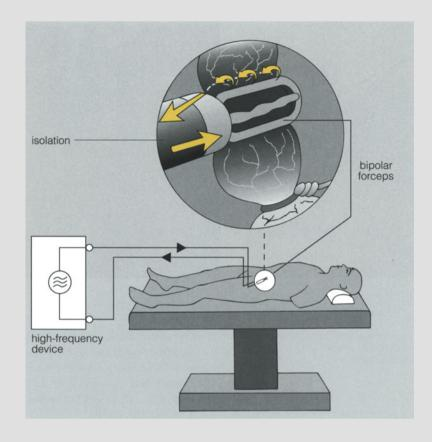
**Fig. 4.8.** Principle of the bipolar HF surgery (e.g. coagulation of adhesions) (*yellow*)
