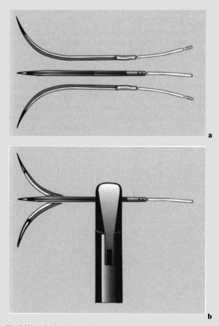
**Fig. 7.27.** a Endo-ski needle which eliminates the problem of needle swivel during laparoscopic suturing by having a triangular shaft. **b** The needle locks in one of three positions within the jaws of a Semm needle holder
