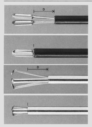
**Fig.2.20.** Hingeless grasping and diathermy forceps (Wolf). To allow the object grasped to remain in the jaws as they are closed, the handle and outer part of the shaft must move a distance (D) towards the tip
