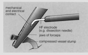
Fig. 4.7. Principle of coaptation coagulation by mechanical compression and electrical energy with jaws of forceps
