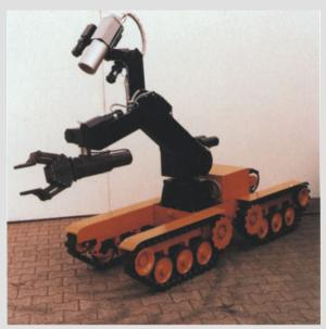
Fig. 27.12. Vehicle with power manipulator
