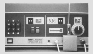
**Fig. 9.18.** Generator for thermostabilized bipolar HF coagulation. The coagulation time *(left)* and coagulation temperature *(center)* can be preset and are displayed by continuous digital readouts. The power in watts *(right)* is microcontroller-regulated when the unit is in the automatic operating mode (circuit diagram, Fig. 9.19)
