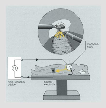
**Fig. 4.3.** Principle of monopolar HF surgery in gallbladder dissection (*yellow*)
