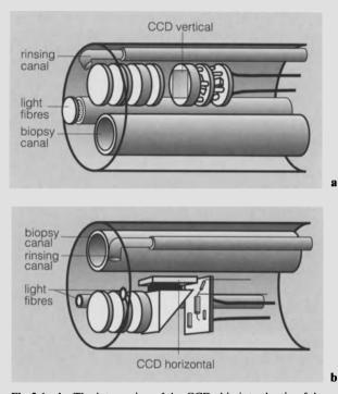
Fig. 2.6a, b. The integration of the CCD chip into the tip of the endoscope. a Olympus, CCD vertical; b Fujinon, CCD horizontal
