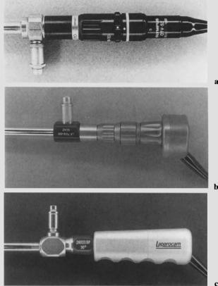
**Fig. 3.4.** a Olympus 1/2''(13-mm) CCD camera coupled glass-toglass to 0° optic. b Baxter-V. Mueller version of arrangement described above employing a 2/3''(17-mm) chip as camera sensor. c Storz Lapcam consolidates a 2/3''(17-mm) CCD sensor and optics ocular within a handgrip, eliminating variable focus
