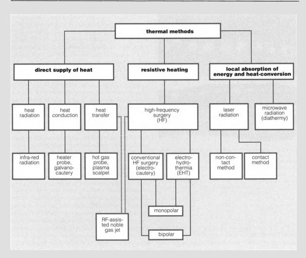
Fig.4.1. Methods for the production of operative-therapeutic heat
