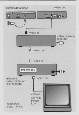
Fig.3.5. Schematic diagram showing connections in video system
