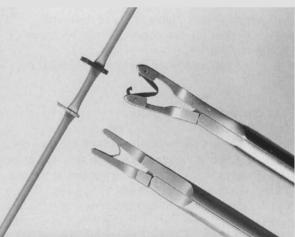
**Fig. 2.27 a, b.** Surgical clips for vessels: **a** Absolock clip (Ethicon) is made of bioabsorbable polydioxanone. For correct clip function the vessel must be free of surrounding tissue for the lock to close without impediment. **b** Metal clips of either stainless steel or titanium are closed by simple plastic deformation, allowing partial or complete closure around a pedicle
