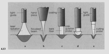
Fig. 4.12. Different transmission systems for laser radiation
