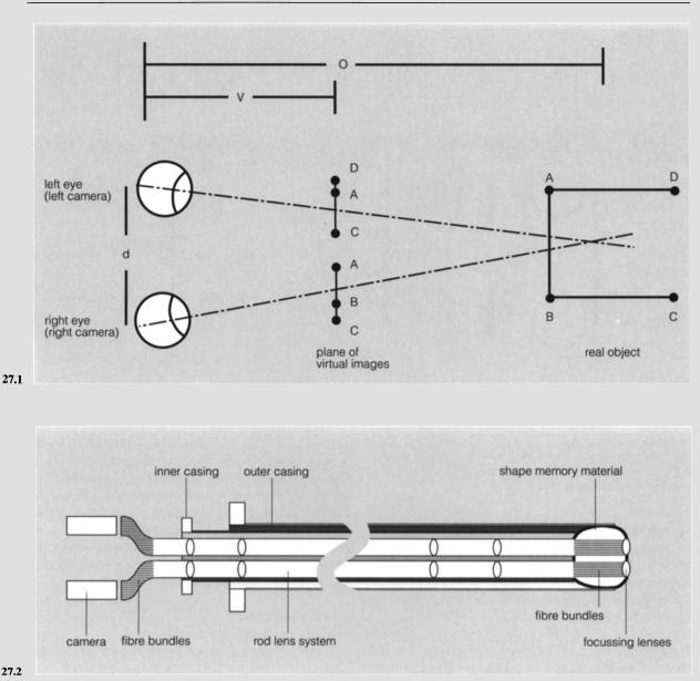
**Fig. 27.1.** Generation of 3D imaging by the oculocerebral system. The two eyes produce images of the real object from different angles due to the interocular distance
