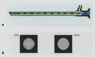
Fig. 2.2. a Longitudinal section of modern rigid endoscope (Panaview, Wolf). Light is reflected at the surfaces of air lenses and transmitted in glass rods. b Distortion of the borders of the image through the endoscope; *old*, conventional lens system; *new*, new lens system using image correction lenses (Olympus, Winter&lbc)
