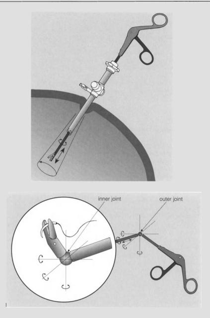
**Fig. 2.1.** a Dimensions of freedom of a conventional instrument in ES. b Concept for a new endoscopic needle holder showing three dimensions of increased freedom. Every movement of the handle is transmitted to the tip of the instrument by the inner and outer ball joints
