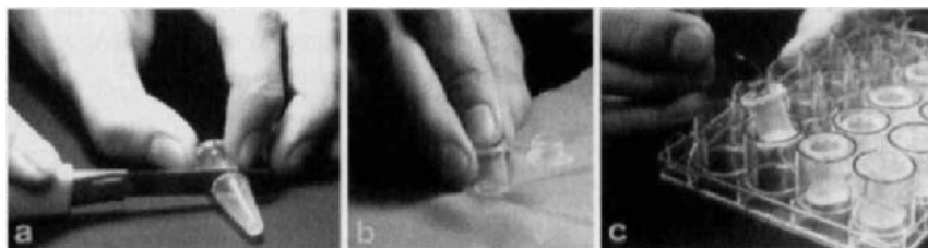
Fig. 3. How to make a basket for cell washing. (a) Cut an Eppendorf tube with a heated knife blade. (b) Push the melted cut end against a nylon mesh. (c) The basket thus made fits into the wells of a 24-well plate.
