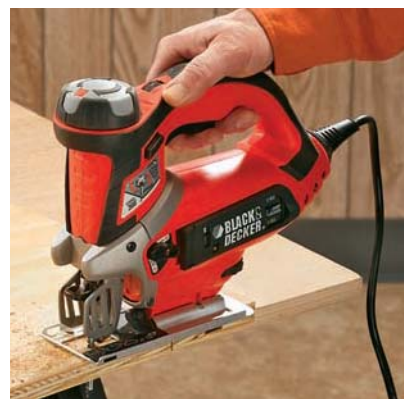
Double-insulated tools have non-conductive plastic bodies to prevent shocks caused by ground faults. Because of these features, double-insulated tools can be used safely with ungrounded receptacles.
