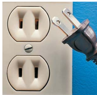
Polarized receptacles have a long slot and a short slot. Used with a polarized plug, the polarized receptacle keeps electrical current directed for safety.
