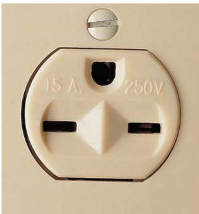
15 amps, 240 volts. This receptacle is used primarily for window air conditioners. It is available as a single unit or as half of a duplex receptacle, with the other half wired for 120 volts.
