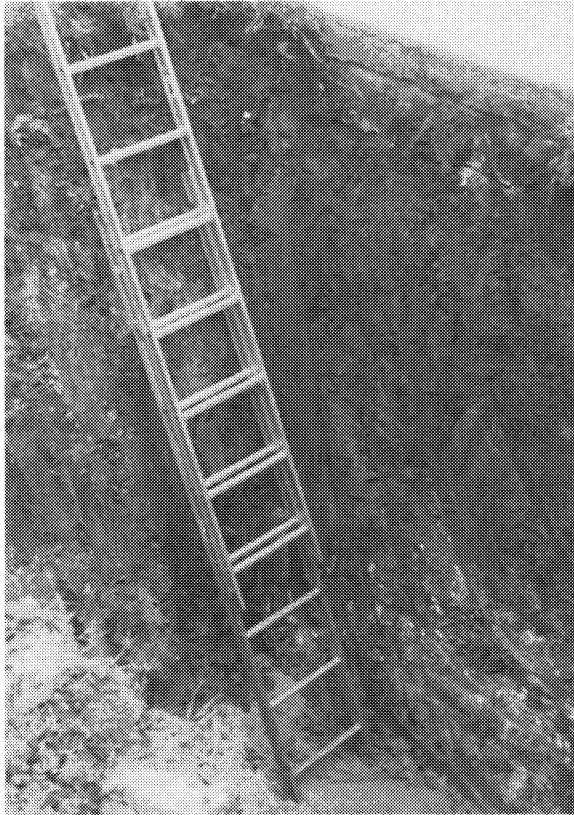
FIGURE 3-4. A test pit in cohesive soil ready for examination.
