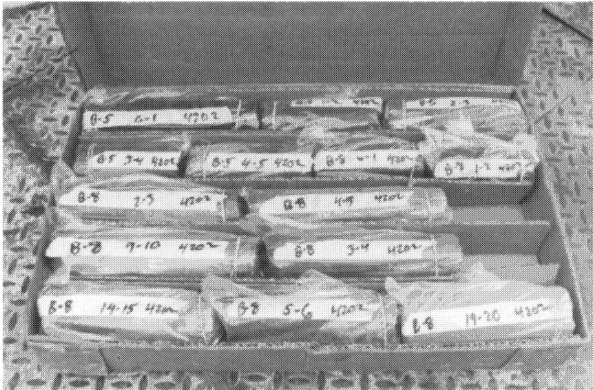
FIGURE 3-8. A box of undisturbed soil samples marked and ready for shipment.
