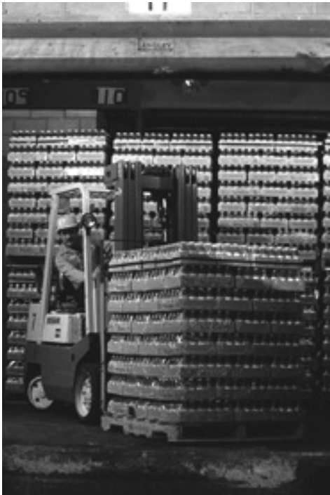
The forklift or fork truck, a common powered industrial truck
