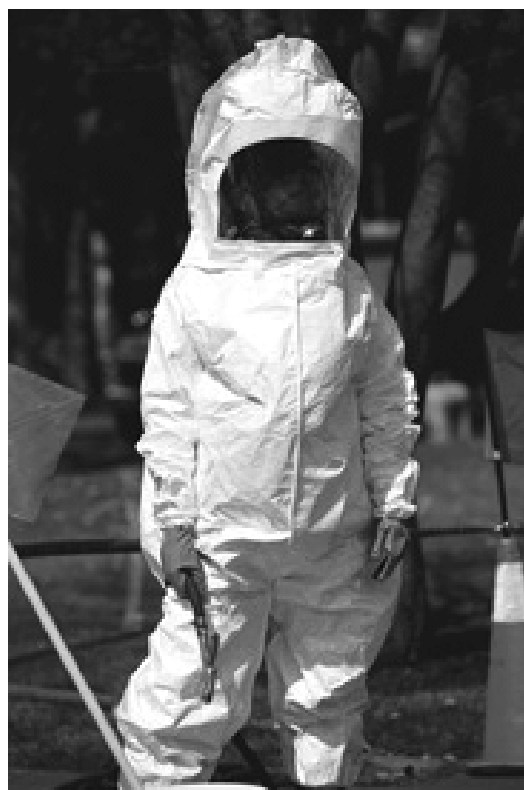
Self-contained ensemble provides whole body protection and breathing air for the user
