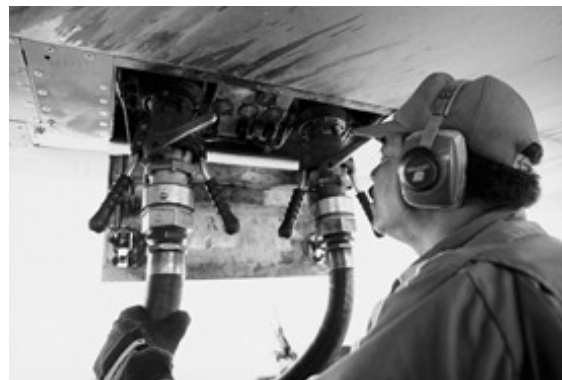
Quick disconnect valves used in the fueling of aircraft allow for quick and safe connection/disconnection of fuel hose lines
